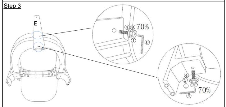
Repeat step 3 to install Back Leg(E). Do Not Fully Tighten the Bolts.
