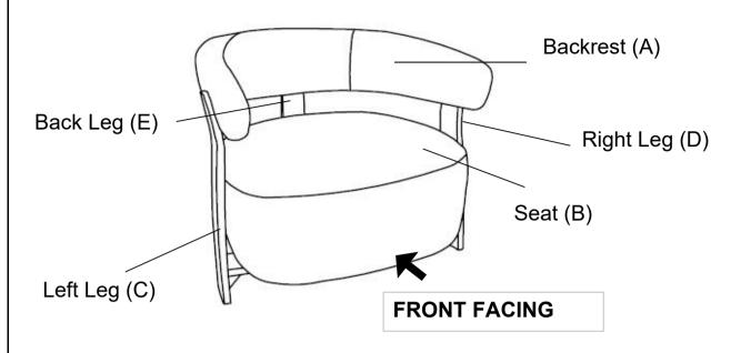
This Chair has multiple parts and may require up to 30 minutes to assemble. To give you an overview of the Chair parts, the above picture is provided to help you put the various parts into perspective. Please read through the instructions below to familiarise yourself with the parts and steps before assembly.
