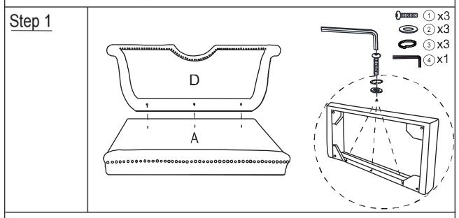
Place the backrest(D) flat on the ground. Align the three holes inside the frame(A) with the three holes at the bottom of the backrest(D). Install and tighten the screws.
