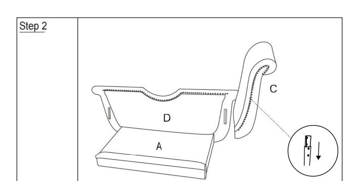
Insert the tab from the left back (C) into the backrest (D)'s tab from bottom to top.
