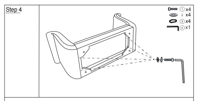
Place the ottoman on the floor. Align the holes on the inner left and right sides of frame (A) with the holes on the back. Insert and tighten the screws.
