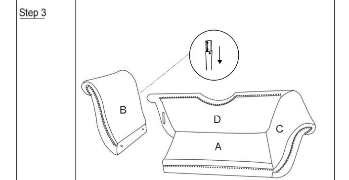
Insert the tab from the right back (B) into the backrest (D)'s tab from bottom to top.
