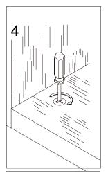
**EN**\_It may be necessary to adjust the hinges so that the doors align. Use the instructions below as a guide.
