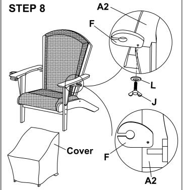
Attach the Glass holder (F) using washer (L) + short butterfly bolts (J).
