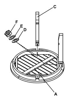
Put the table top (A) face down on clean flat surface. Attach 2 pcs legs (C) to the table top (A) and secure each leg with washer (D), spring washer (E) and nuts (F). Do not fully tighten all nuts yet.
