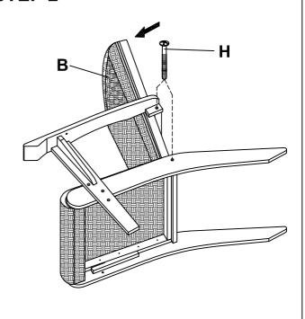
Attach left side frame (A2) into Seat (C). secure with 1" bolts (H).
