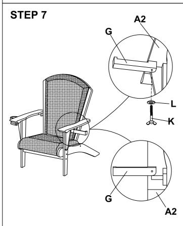
Attach the cell phone holder (G) using washer (L) + long butterfly bolt (K) for the Cell phone holder (G). The cell phone holder (G) can only be installed on the left side frame (A2)
