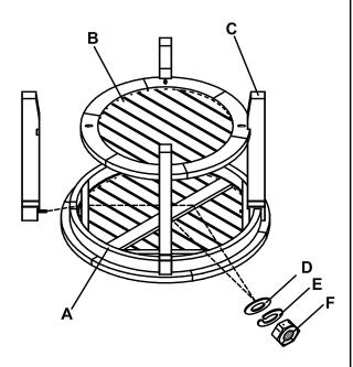
Attach the tray (B) to the legs (C). Attach the other legs (C) into the table top (A) and tray (B), as diagram shown. Secure the legs (C) to table top (A) with washer (D), spring washer (E), and nuts (F).
