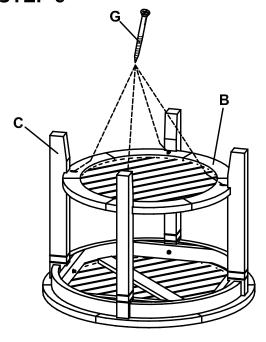
Secure the tray (B) with 1 1/2" screws (G). Make sure all parts are correctly connected and tighten all nuts and screws completely using phillips screwdriver and wrench.
