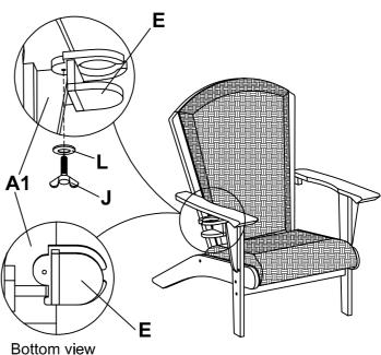
Attach the bottle holder (E) using washer (K) + short butterfly bolts (J) and washer (L).
