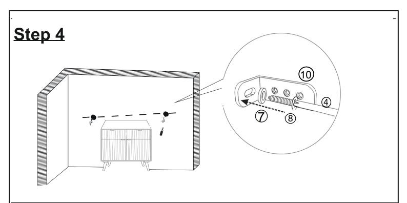
Attach Brackets (10) to Wall Plugs (11) using Wall Plug Screws (8) Washer (7) with Screwdrivers (4)
