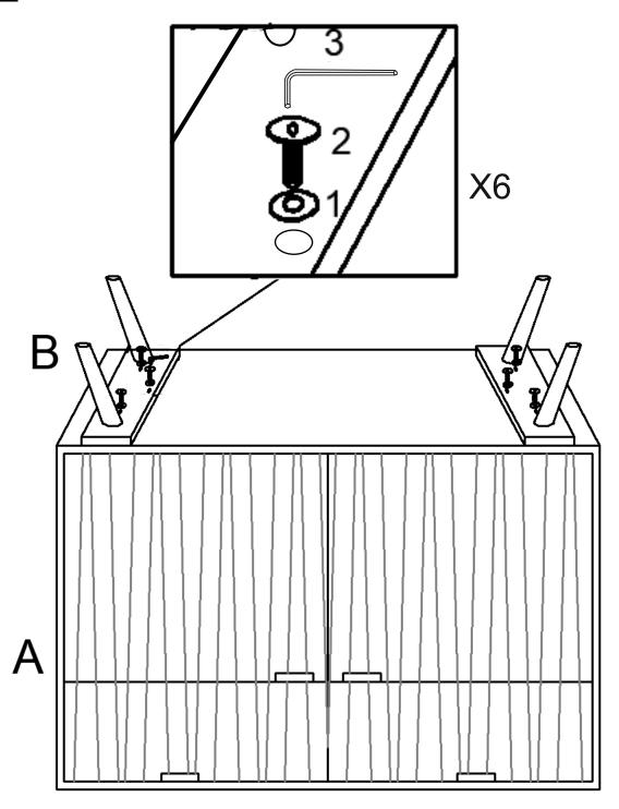
With assistance from your adult partner, place the Cabinet (A) face down as picture on clean surface. As shown in above picture, attach Leg (B) to Cabinet (A) using Washer (1), Bolt(2) with Allen Wrench (3).
