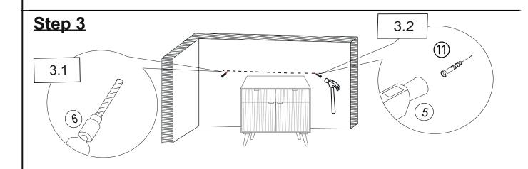
3.1) Drill two holes on wall at same height as Bracket (1) on Cabinet (A) with Power Drill (6).
