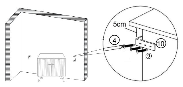
Move Cabinet to the wall, customer can one of 3 holes for assembly same as other side.
