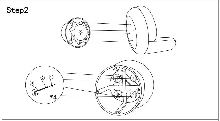
Align the four holes on the turntable above the single chair leg bucket (B) with the four holes on the bottom of the single chair body (A), and place the spring washer (1) on the bolt (2) and lock it with an allen key (3)
