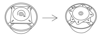
Rotate the turntable above the single chair leg bucket(B) by 45  $^{\circ}$
