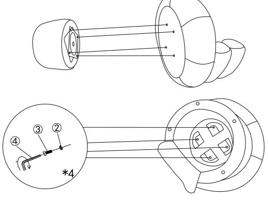
Align the four holes on the turntable above the single chair leg bucket (B) with the four holes on the bottom of the single chair body (A), and place the spring washer (2) on the bolt (3) and lock it with an allen key (4)
