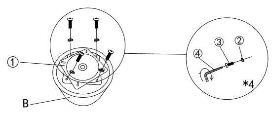
Align the 4 holes under the turntable (1) with the 4 holes on the single chair leg bucket (B), and place the spring washer (2) on the bolt (3) and lock it with an allen key (4)
