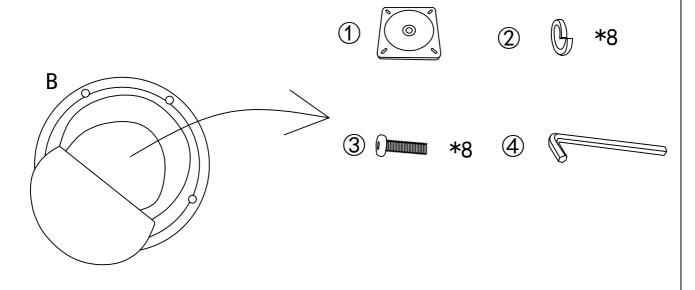
Open the bottom zipper of the single chair leg bucket (B), take out the Turntable (1), spring washer (2), bolt (3), and allen key (4)
