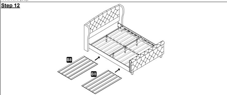
Place the slat (B8) on the assembled bed frame and paste the magic strip into place.
