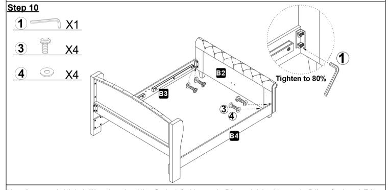
Use allen wrench (1), bolt (3) and washer (4) to fix the left side panel (B3) and right side panel (B4) on footboard (B2)
