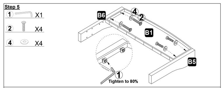
Align the hole of the head of the headboard (B1) with the hole inf the right wing panel (B5) and left wing panel (B6), and then fix it with allen wrench (1), bolt (2), washer(4).
