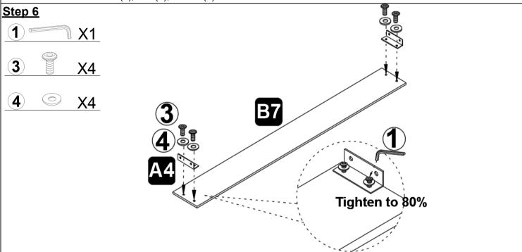
Use allen wrench (1), bolt (3) and washer (4) to secure the angle iron (A4) to the baffle under the head of the bed (B7) at the head of the bed.
