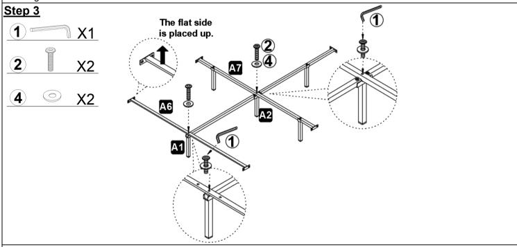
Use the allen wrench (1), bolt (2), washer(4) to fix the bedside connecting rod (A6) to the front and back support foot (A1) as shown in the figure, and the middle connecting rod (A7) to the middle support foot (A2).
