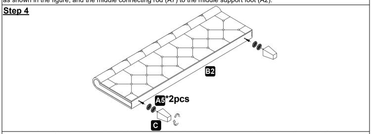
The plastic feet (C) and the non-slip pads (A5) are fixed clockwise at the corresponding position of the end of the footboard (B2).
