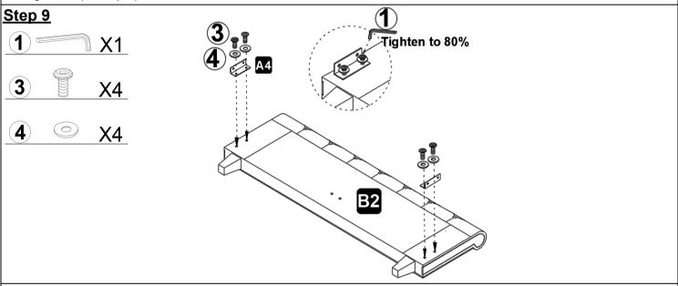
Use the allen wrench (1), bolt (3), washer (4) to fix the angle iron (A4) to the footboard (B2).
