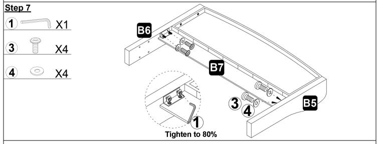
Use allen wrench (1), bolts (3) and Washers (4) to fix the the baffle under the head of the bed (B7) on the head of the bed and then the right wing panel (B5) and left wing panel (B6).
