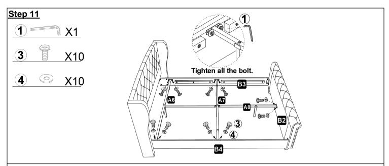
Use allen wrench (1), bolt (2) and washer (4) to fix the left and right ends of the bedside connecting rod (A6) and the middle connecting rod (A7) on the left panel (B3) and the right panel (B4), and fix the bed tail connecting rod (A8) to the footboard (B2).
