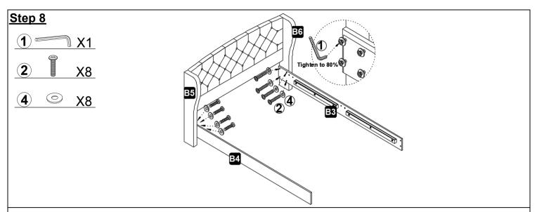
Use allen wrench (1), bolt (2), washer(4) to fix the right wing panel (B5) and left wing panel (B6) on the left side panel (B3) and right side panel (B4).
