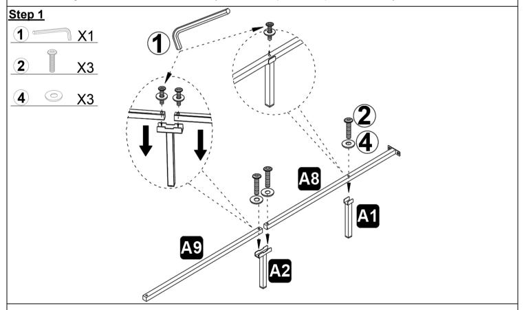
As shown in the figure, use allen wrench (1), bolt (2), washer(4) to fix the front and rear connecting rods center connecting rod(A9) and bed tail connecting rod(A8) to the middle support foot (A2) and front and back support foot (A1).
