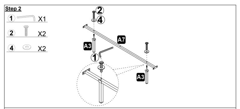
Use allen wrench (1), bolt (2) and washer (4) to fix the middle connecting rod (A7) on the side middle foot (A3) as shown in the figure.
