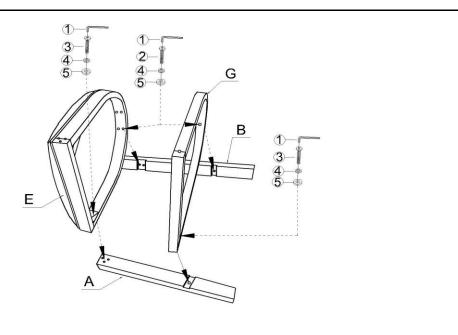
Use the Allen Wrench (①), bolts (②) or (③), spring washers (④) and flat washers (⑤) to install the Seat cushion (E), Bottom frame (G) and two legs(A and B) as shown in the figure above.
