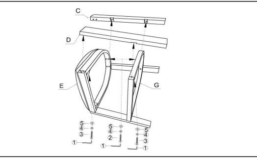
Use the Allen Wrench (①), bolts (②) or (③), spring washers (④) and flat washers (⑤) to install the Seat cushion (E), Bottom frame (G) and two legs(C and D) as shown in the figure above.
