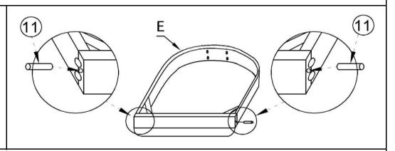
As shown in the picture, place the Wooden tenon (11) in the wooden tenon hole on the side of the Seat cushion (E).
