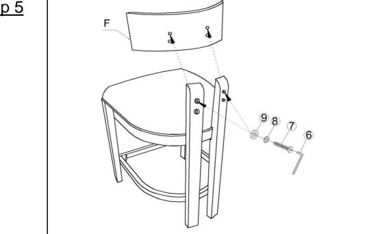
Install the Chair Backrest (F) as shown in the figure above using the Allen Wrench (©), bolts (⑦), spring washers (®) and flat washers (®).
