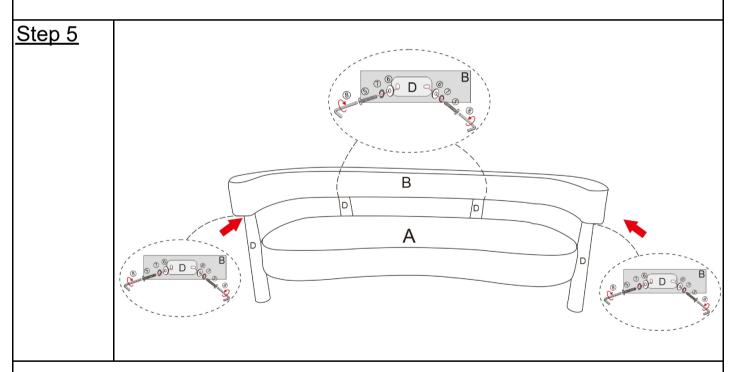
After aligning the holes of Leg (D) with those of Backrest (B), tighten Gaskets (③), Spring Shims (⑦) and Single Head Screw (⑤) in sequence from the bottom using Allen Wrench (⑧). This step involves tightening Single Head Screw (⑤) Repeat this procedure eight times.
