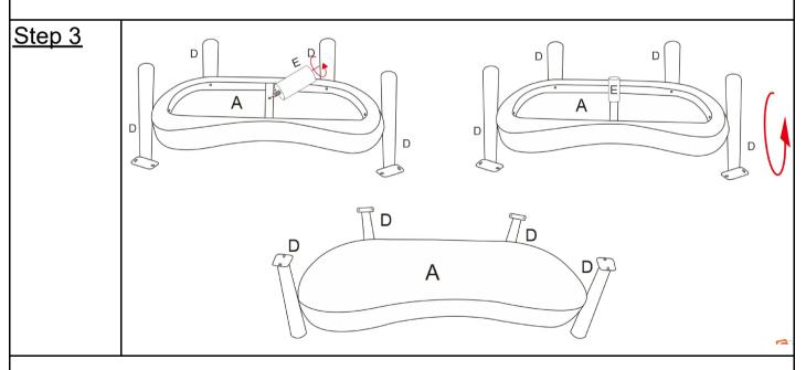
Align Middle Leg (E) with the central hole in Seat Board (A), screw it into the hole, and tighten Middle Leg (E). Then turn Seat Board (A) over to its front side.
