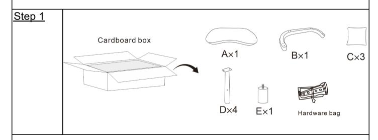
Remove items Seat Board (A), Backrest (B), Back Cushion (C), Leg (D), Middle Leg (E) and the hardware kit from the cardboard box, and place them on a clean, scratch-free surface.
