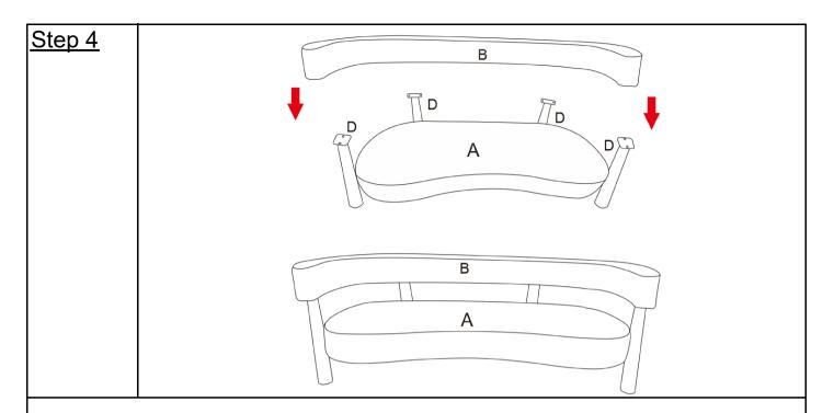
Place Backrest (B) horizontally upon Leg (D), aligning the holes in Backrest (B) with those in Leg (D).
