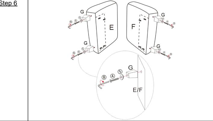
Align Sofa Wooden Legs (G) with the holes at both ends of the bottom of Right Armrest (F) and use Allen Wrench (®) to tighten the Gaskets (⑤), and Single Head Screw (4) in sequential order.
