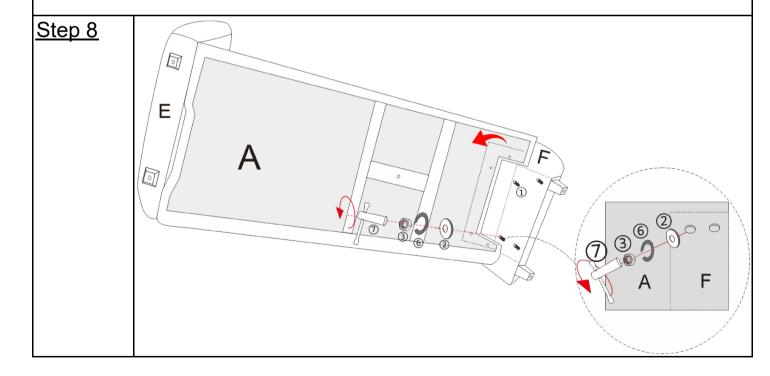
Place Right Armrest (F) and Seat Board (A) vertically on the ground, put Right Armrest (F) and Seat Board (A) close together, and lock Gaskets (2), Spring Shims (6), and Nut (3) on Double Headed Screw (1) with Wrenches (7), and tighten the screws in this step.
