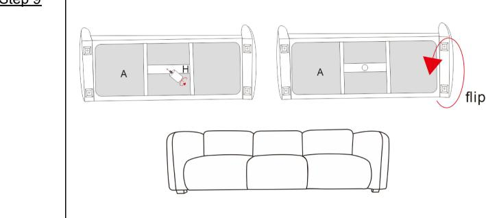
Fit Middle Leg (H) in the centre of the bottom of Seat Board (A) and flip the whole couch back over.
