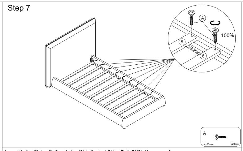
Assemble the Slats with 2pre-holes (6) to the bed Sides Rail (R)(3). Use screw A
