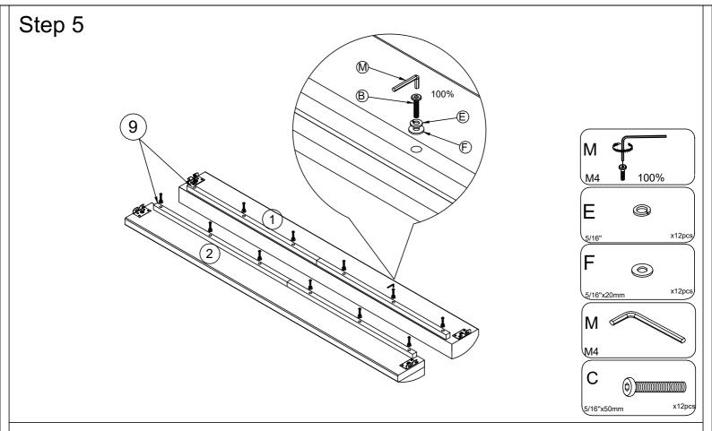
Attach the Support Rail (9) to the Side Rail (3) and the Side Rail (4). By using the Bolts (C), the Flat Washer(F) and the Lock Washer(E) with M4 Allen Wrench(M)
