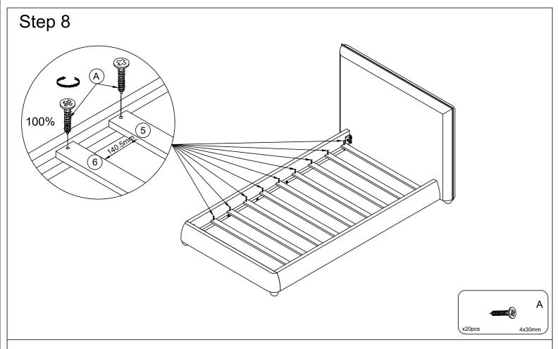
Assemble the Slats with 2pre-holes (6) to the bed Sides Rail (L)(4). Use screw A
