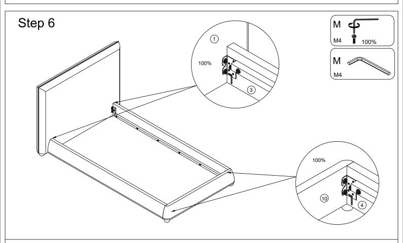
Attach the Side Rail (3) to the Headboard(R)(1)and the Side Rail (4) to the Headboard(L)(2),by using M4 Allen Wrench (M) to tighten the Bolts (B). Then attach the Footboard (10) to the Side Rail (3) and the Side Rail (4) by using M4 Allen Wrench (M) to tighten the Bolts (B).(Note: the direction of the Metal pad is down)
