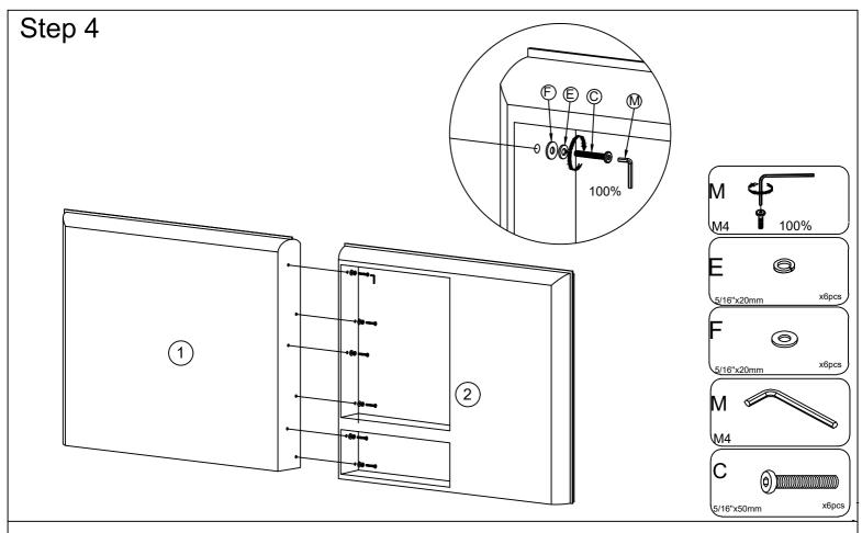
Use the Bolts (C), Lock washer (E) and Flat washer (F) to connect the Headboard(R)(1) and the Headboard(L)(2) then tighten with Allen Wrench (M)
