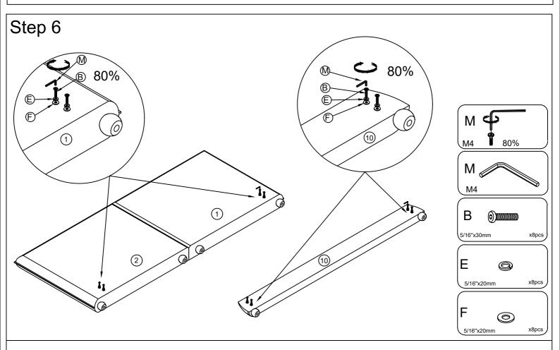
Use Bolts (B) and Lock Washer (E) with Flat Washer (F). Then attach 1/2 Bolts (B) to the Headboard(R)(1), Headboard(L)(2) and Footboard (10).
