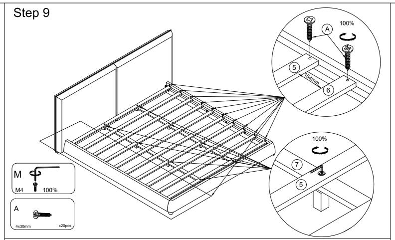
Assemble the Slats with 4pre-holes (5)and the Slat with 2pre-holes to the bed Sides Rail (1) and (2). Use screw A Finally, use the M4 Allen Wrench (M) to tighten the Bolts (D) 100%
