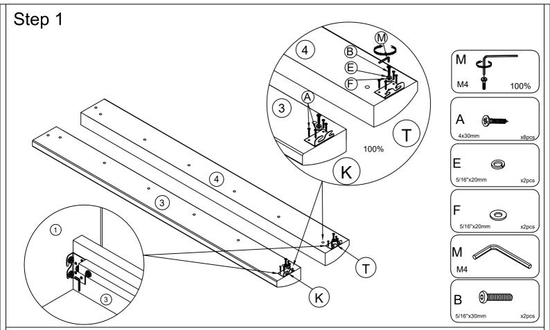
Attach the Metal pad (K) to the Side Rail (R) (3), attach the Metal pad (T) to the Side Rail (L) (4). By using the Bolts (B) and Flat Washer (F) with the Lock Washer (E) and Screw (A) to connect the Metal pad and the Side Rail Note: The Metal pad hook is facing down and this place is connected to the Headboad(R) (1) and Headboard (L)(2).
