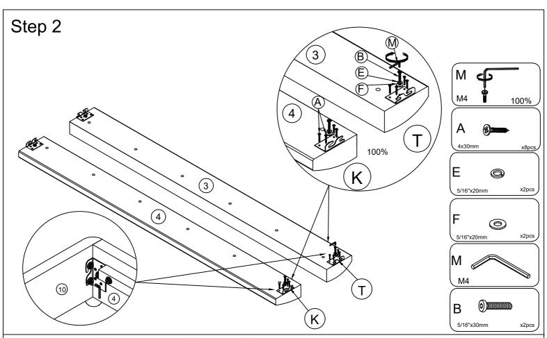
Use the Metal pad (T) to attach to the Side Rail (3), use the Metal pad (K) to attach the Side Rail (4). By using the Screw (A) and the Bolts (B) with M4 Allen Wrench (M) to connect the Metal pad and the Side Rail Note: The direction of the Metal Pad and this place is connected to the Footboard (10).
