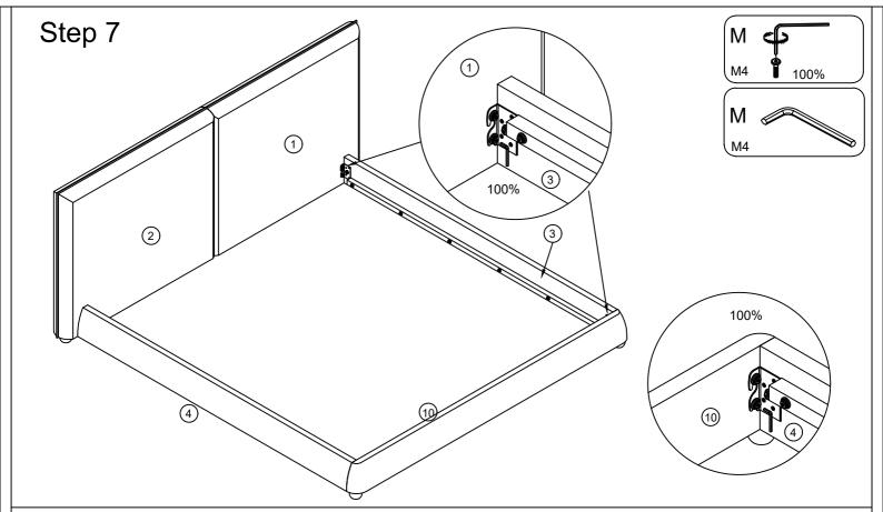
Attach the Side Rail (3) to the Headboard(R)(1)and the Side Rail (4) to the Headboard(L)(2),by using M4 Allen Wrench (M) to tighten the Bolts (B). Then attach the Footboard (10) to the Side Rail (3) and the Side Rail (4) by using M4 Allen Wrench (M) to tighten the Bolts (B).(Note: the direction of the Metal pad is down)
