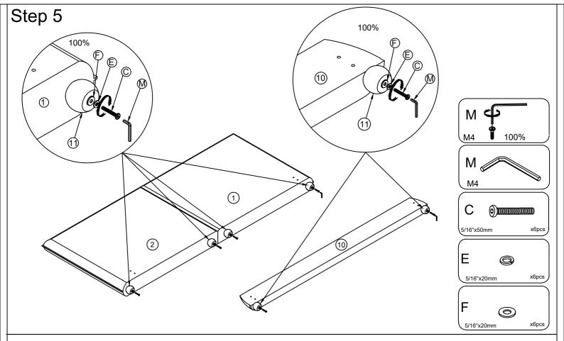
Attach the Bed Legs(11) to the Headboard (R)(1), Headboard(L)(2) and the Footboard (10). By using the Bolts (C), the Flat Washer(F) and the Lock Washer(E) with M4 Allen Wrench(M)
