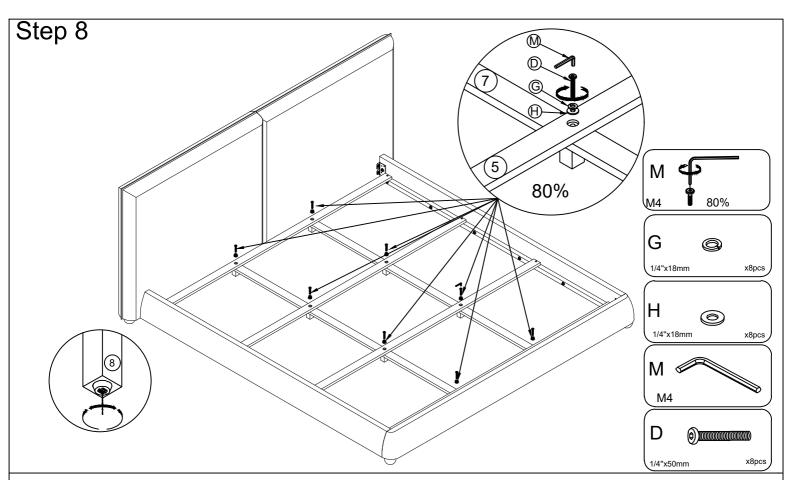
Align the assembly position on the Middle Support Bar (7) with the Center Support Leg (8) and the Slats with 4 pre-holes (5). Then attach the Slats with 4pre-holes (5) and the Middle Support Bar (7) to the Center Support Leg (8).By using the Bolts (D),Lock Washer (G) with Flat Washer (H) with M4 Allen Wrench (M).
