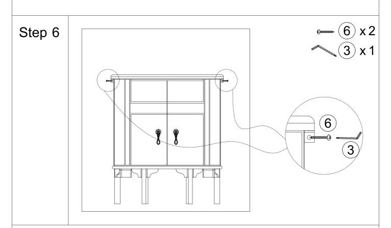
Align with the expansion plug (⑤),install the short side of anti-tip wall bracket (④) on the wall with long screw (⑥) using screwdriver(③). Ensure the brackets are level and aligned with the wall before drilling.
