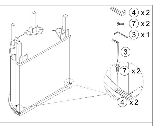
Attach long side of anti-tip wall bracket (4) at the 2 sides of the cabinet top with short screw(7) using screwdriver (3).
