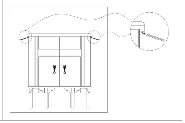
Place the cabinet against the wall. Mark the position for extension plug.
