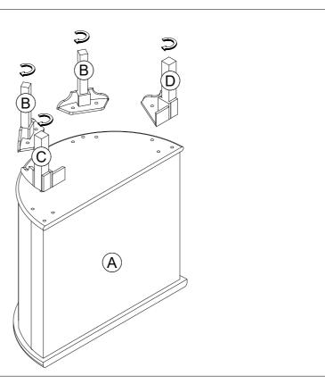
Align middle leg(B), left leg(C), right leg(D) with cabinet body(A).
