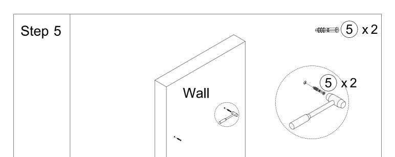
Drill holes on the wall in marking position, Insert the expansion plug(5).
