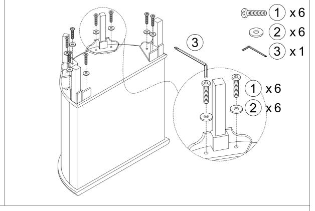
Attach middle leg(B) $\setminus$  left leg(C) $\setminus$  right leg(D) to cabinet body(A) with bolt(1) and washer (2) using screwdriver (3).
