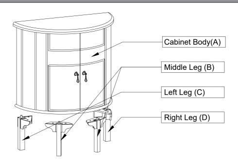
This cabinet has multiple parts and may require up to some 20 minutes to assemble. To give you an overview of the cabinet parts, the above picture is to help you put the various parts into perspective. Please read through the instructions below to familiarise yourself with the parts and steps before assembly.
