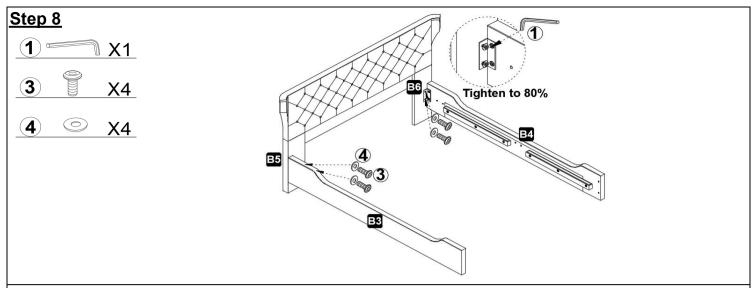
Use Allen wrench (1), Bolt (3) and Washer (4) to fix the bed side (B3&B4) on the bed post (B5&B6).
