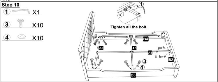
Use hex wrench (1), bolt (3) and washer (4) to fix the left and right ends of the bedside connecting rod (A5) and the middle connecting rod (A6) on the left panel (B3) and the right panel (B4), and fix the bed tail connecting rod (A8) to the end of the bed (B2).
