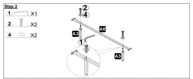
Use Allen wrench (1), Bolt (2) and Washer (4) to fix the middle connecting rod (A6) on the side middle foot (A3) as shown in the figure.
