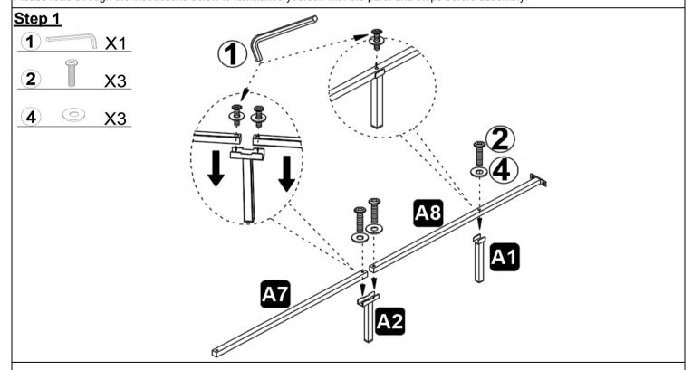
Use Allen wrench (1), Bolt (2), Washer (4) to fix the front and rear connecting rods (A7&A8) to the metal foot (A2&A1) as shown in the figure.
