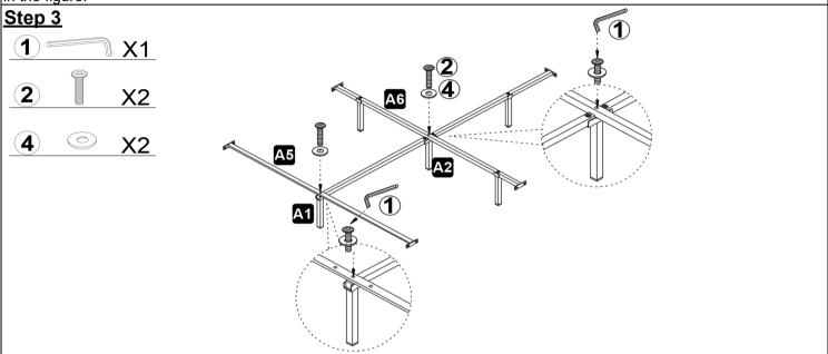
Use the Allen wrench (1), Bolt (2), Washer (4) to fix the front connecting rod (A5) to the front middle foot (A1) as shown in the figure, and the middle connecting rod (A6) to the middle foot (A2).
