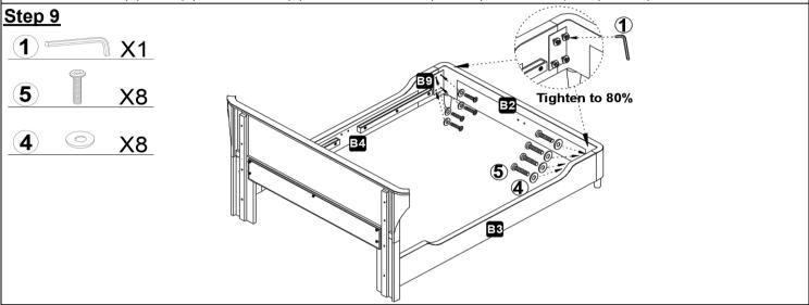
Use Allen wrench (1), Bolt (5) and Washer (4) to fix the bed tail (B2) and the bed side plate (B3&B4) with metal plates (B9).
