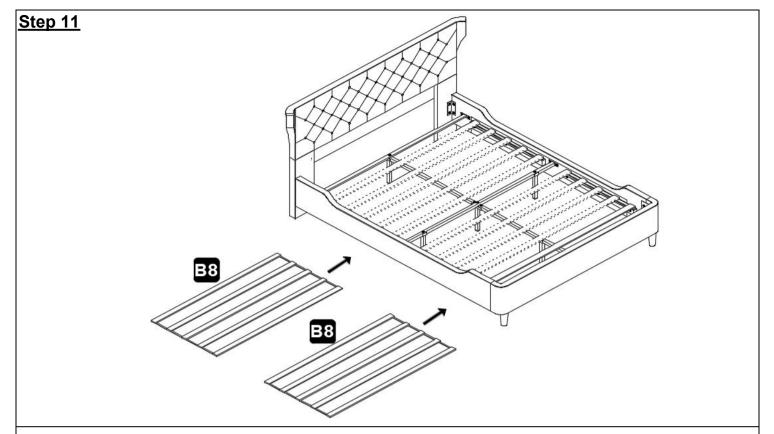
Place the bed frame strip (B8) on the assembled bed frame and paste the magic strip into place.
