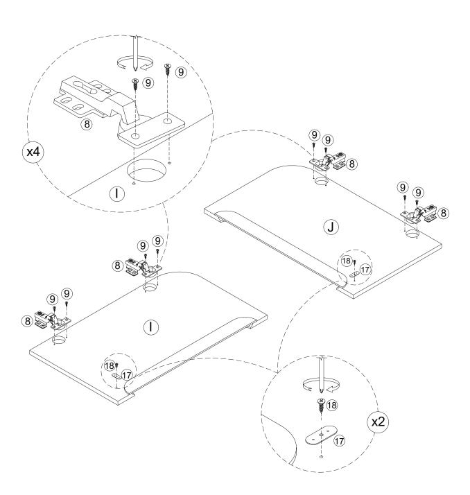
It's all coming together! Secure the doors to the unit by the Hinges using the M4 x 14mm Screws (9).
