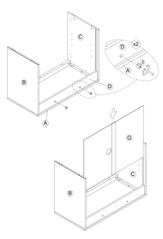
Insert the Wooden Dowels (3) into the Side Panel (Right) (C) & Side Panel (Left) (B), then attach it to the Bottom Panel (F) using the Camlocks (2).
