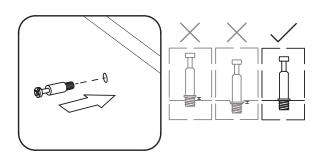
Next, you will fit the proper hole on the edge of the associated joining panel over the cam bolt.
