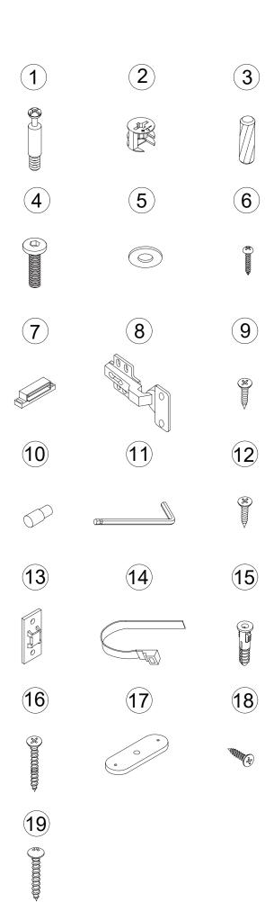
Let's get this thing fired up! Start by putting Cam Bolts (1) into the Top Panel (A), Side Panel Left (B), Side Panel Right (C), and Bottom Panel (F), in the holes indicated below.
