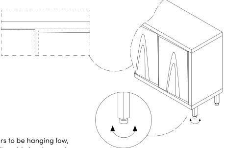
If the left door appears to be hanging low, you can adjust the adjustable leveler on the front left until the door is better aligned.
