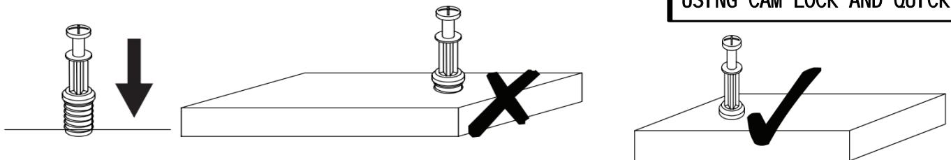
**EN-QUICKFIT:** Tighten quickfit until shoulder is flush with panel. Do not overtighten or undertighten.
