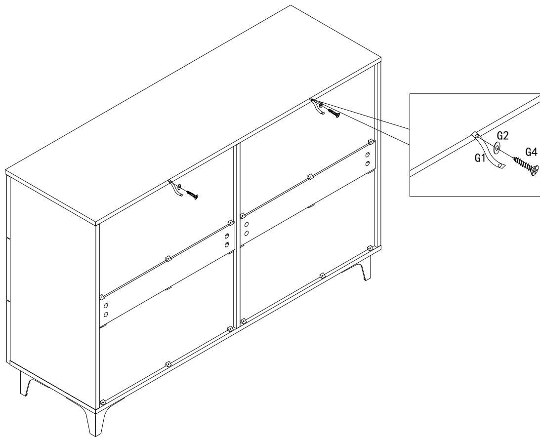
**Warning:** This product is equipped with an anti-tilt device. Please be sure to install this device to prevent unnecessary injuries caused by tipping.
