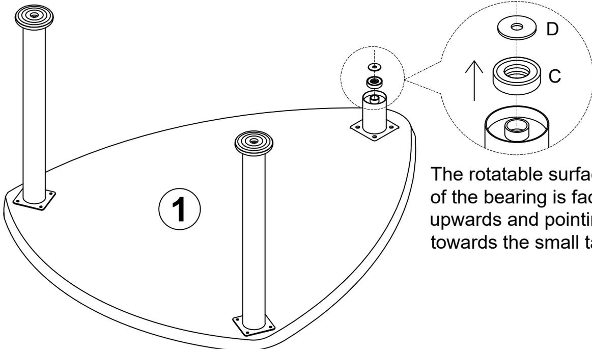
The rotatable surface of the bearing is facing upwards and pointing towards the small table.
