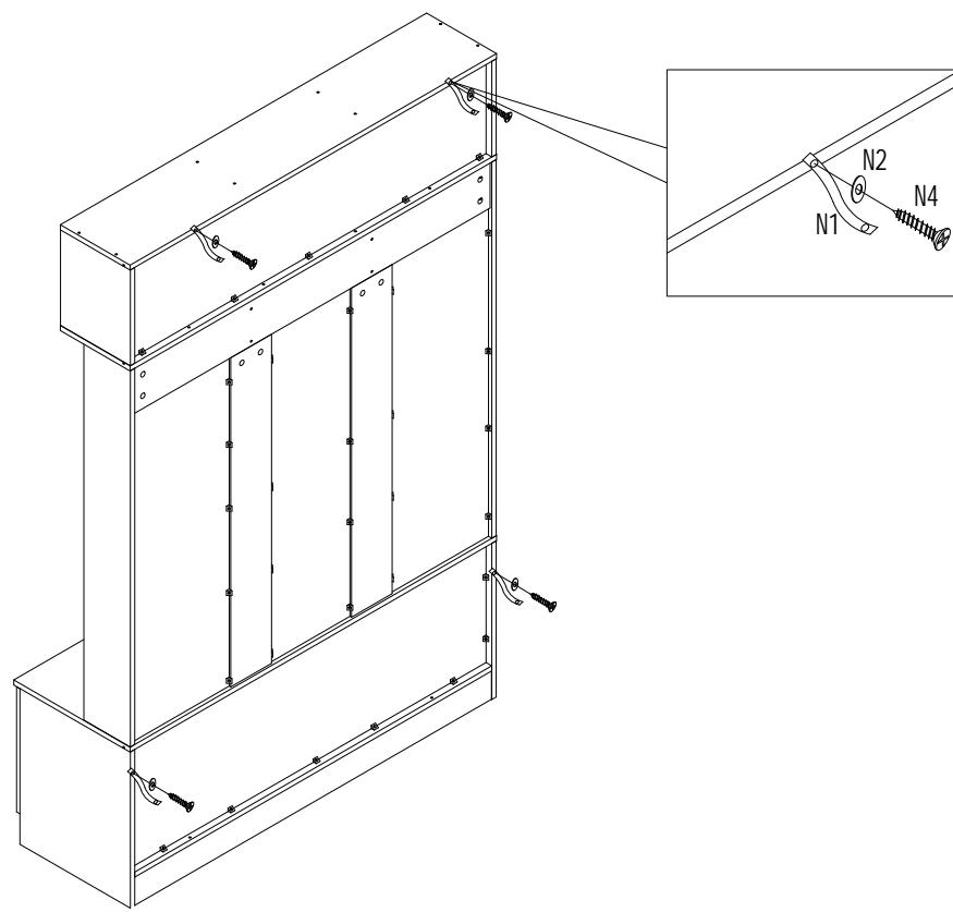
**Warning:** This product is equipped with an anti-tilt device. Please be sure to install this device to prevent unnecessary injuries caused by tipping.
