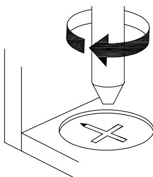
**EN**\_Turn cam lock clockwise to tighten.
