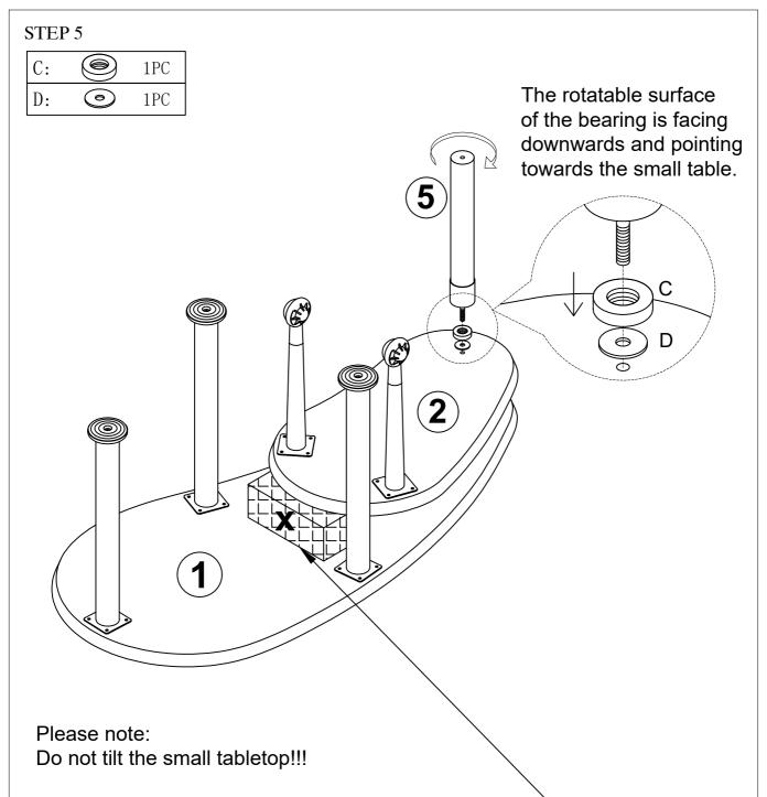
Before installing the leg ⑤, please place a support item **X** on the edge of the small tabletop to ensure that the small tabletop is parallel to the large tabletop, and the hole of the small tabletop is perpendicular to the center axis of rotation, so that the screws of the leg can be installed smoothly.
