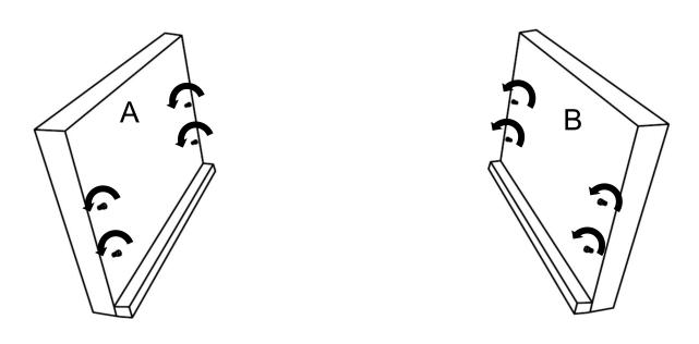
**Step 2**: Attach the **Left Hingers(M)** and **Right Hingers (N)** to the **Front Panel(D)** and **Back Panel(C)** with **Bolt(K)** and **Screw(L)** at the right position like picture shows
