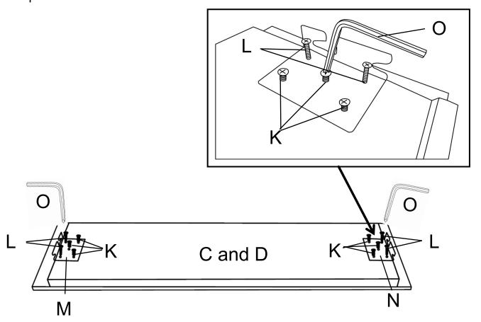
Step 3: Connect the Back Panel(C)/Front Panel(D) and Left Panel(A)& Right Panel(B) together and then secured with Allen wrench(O)
