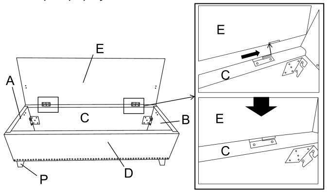
**Step 6**: Connect the **Left Hinge(G)** to the **Left Arm(A)** and **Bench Top(C)** and the **Right Hinge(H)** to the **Right Arm(B)** and **Bench Top(C)** with **Bolt(J)** and **Allen Wrench(K)**.
