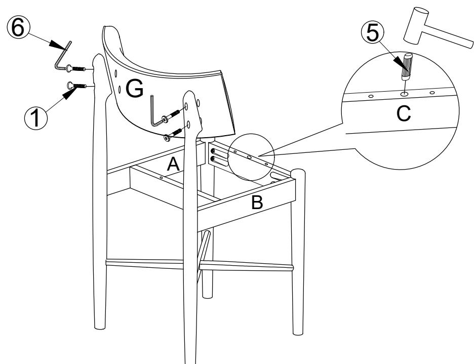
Place Back Cushion (G) to Side Leg (A&B) With Hardware JCBC Screw (1) using the Allen Key (6) and fit the Wood Dowel (5) into the Front Rail (C) as shown in picture.
