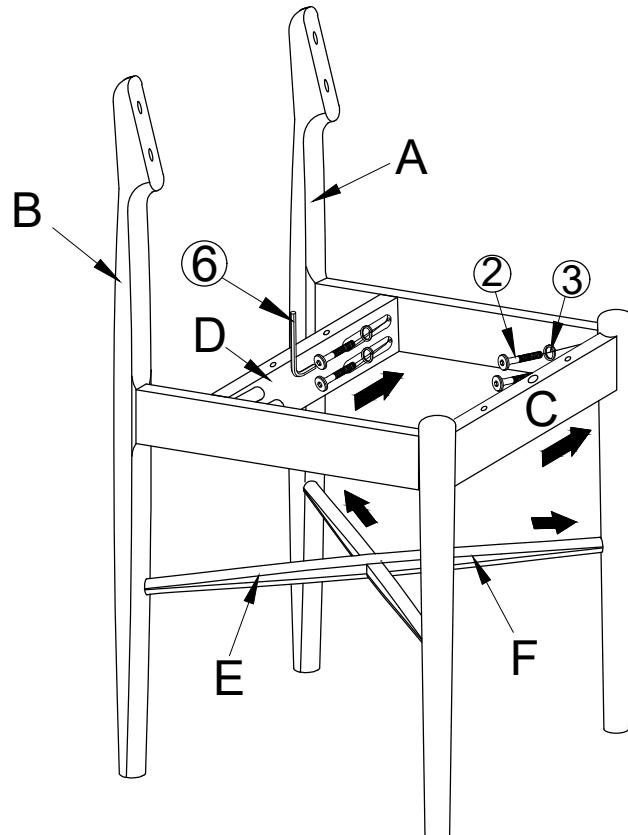
Place Front Rail (C) & Back Rail (D) to Side Leg-Left (A) With Hardware JCBC Screw (2) + Spring Washer (3). Using the Allen Key (6) .And place Stretcher (E&F) into the hole of Side Leg Left (A) as shown in picture.
