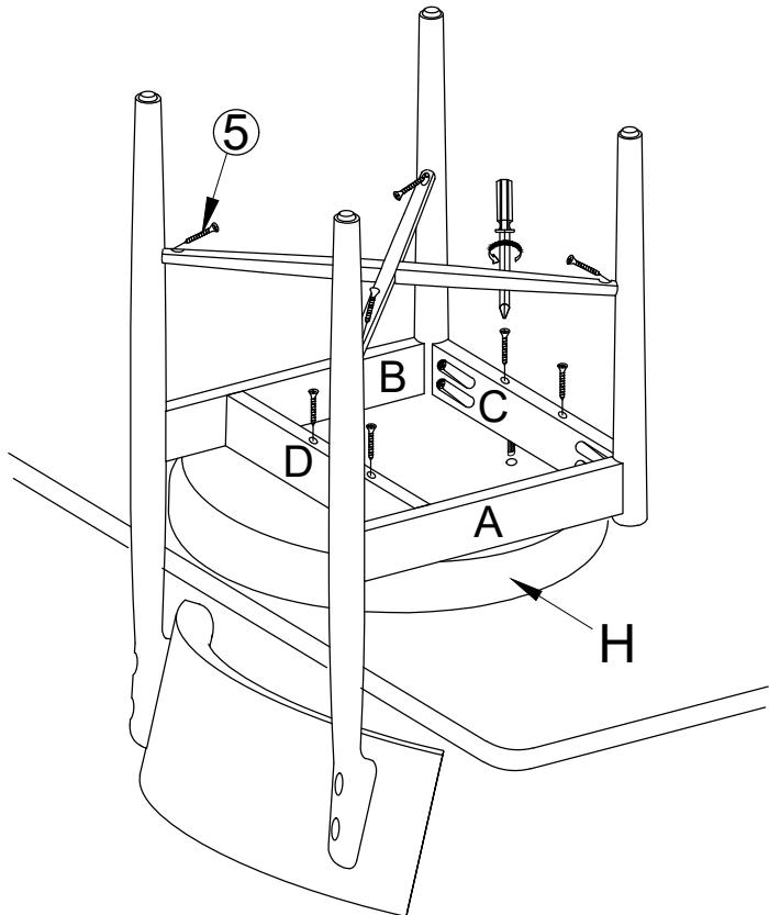
Fit the cushion seat (H) hole to wood dowel and fit cushion seat (H) & Stretcher (E&F) with CSK Screw (5) using the screwdriver as shown in picture.
