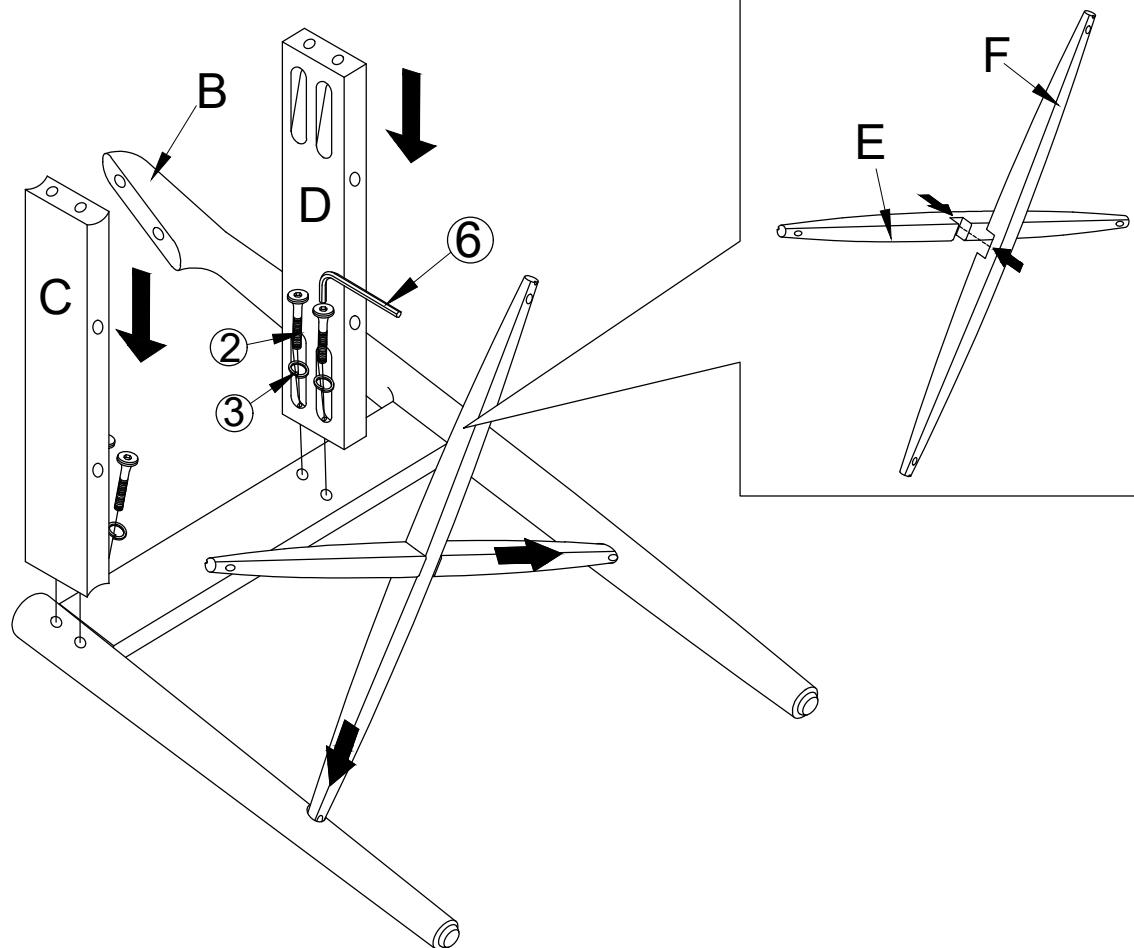
Place Front Rail (C) & Back Rail (D) to Side Leg-Right (B) With Hardware JCBC Screw (2) + Spring Washer (3) using the Allen Key (6). Put Stretcher (E&F) together as shown in picture and place it into the hole of Side Leg Right (B) . Rotate Stretcher (E&F) if the hole doesn't fit.
