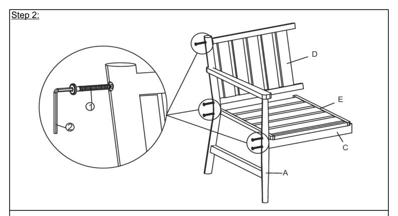
With the help of your adult partner, insert the tenons of Backrest Panel (D), Seat Panel (E) and Front Support Bar (C) into the mortises of Left Leg Panel (A) as shown above.
