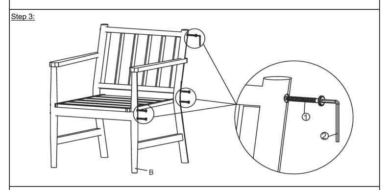
With the help of your adult partner, insert the tenons of Backrest Panel (D), Seat Panel (E) and Front Support Bar (C) into the mortises of Right Leg Panel (B) as shown above.
