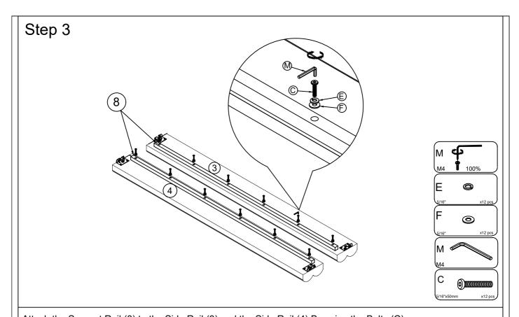
Attach the Support Rail (8) to the Side Rail (3) and the Side Rail (4).By using the Bolts (C), the Flat Washer(F) and the Lock Washer(E) with M4 Allen Key(M)
