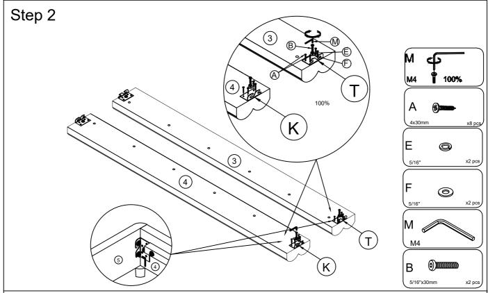
Attach Metal pad (T) to the Side Rail (3), attach Metal pad (K) to the Side Rail (4), by using the Bolts (B), Flat Washer (F), Lock Washer (E) and Screw (A) with Allen Key (M). Note :The direction of the Hinge and this place is connected to the Footfoard (5).
