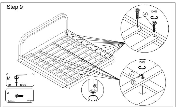
Attach the Slats with 4pre-holes and the Slat with 2pre-holes to the bed Sides Rail (1) and (2). Use screw A Finally, use the M4 Allen Wrench (M) to tighten the Bolts (D) 100%. Adjustable leveling foot of Center Support Legs.
