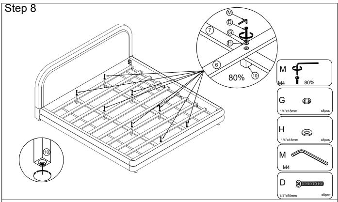
Align the assembly position on the Middle Support Bar (7) to the Center Support Leg (10) and the Slats with 4pre-holes (6). Then attach the Slats with 4pre-holes (6) and the Middle Support Bar (7) to the Center Support Leg (10).By using the Bolts (D),Lock Washer (G) with Flat Washer (H) with M4 Allen Wrench (M).
