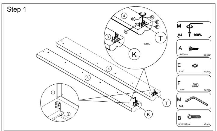
Attach the Metal pad (K) to the Side Rail (R) (3), attach the Metal pad (T) to the Side Rail (L) (4), by using the Bolts (B), Flat Washer (F), Lock Washer (E) and Screw (A) with Allen Key (M). Note: The hinge hook is facing down and this place is connected to the Headboard Storage (2).
