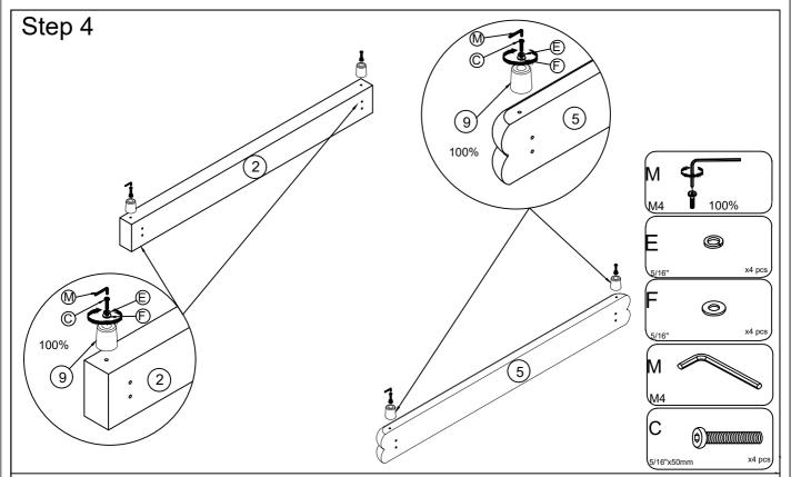
Attach 2 Bed Legs (9) to the Headboard Storage(2) and 2 Bed Legs(9) to the Footboard (5), by using Bolts (C), Lock Washer (E), Flat Washer (F) with Allen Key (M).
