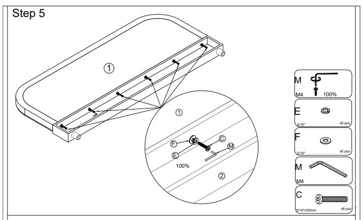
Attach the Headboard(1) to the Headboard Storage(2). By using the Bolts (C), the Flat Washer(F) and the Lock Washer(E) with M4 Allen Key(M)
