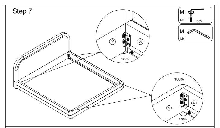
Attach the Side Rail (3) and the Side Rail (4) to the Headboard Storage(2),by using Bolts (B) with M4 Allen Wrench (M). Then attach the Footboard (5) to the Side Rail (3) and the Side Rail (4) by using Bolts (B) with M4 Allen Wrench (M). Note: the direction of the Metal pad is facing down.
