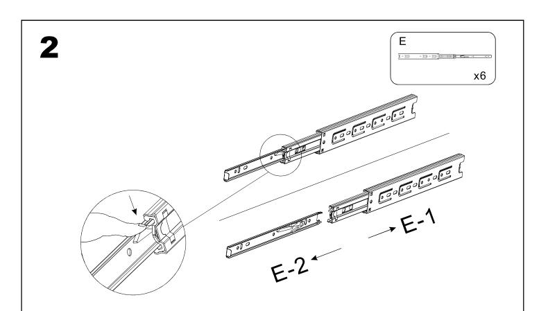
• Press the button and extend the slide slowly. Then separate it with the release latch. Repeat these steps for the other slides.
