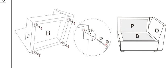
Lay Right Seat Board (B) flat, align Leg (M) with the holes at the bottom of Right Seat Board (B), and use Allen Wrench (6) to tighten Single Head Screw (1). This step tightens Single Head Screw (1).
