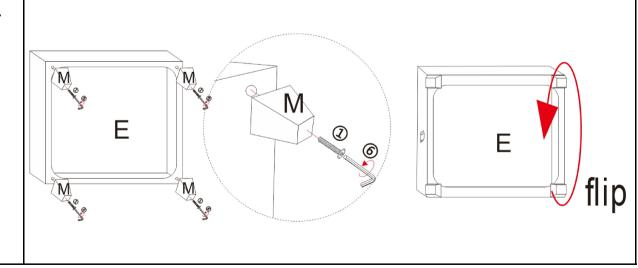
Lay Footrest (E) flat, align Leg (M) with the hole at the bottom of Footrest (E), and use Allen Wrench (6) to tighten Single Head Screw (1). This step will completely tighten Single Head Screw (1).
