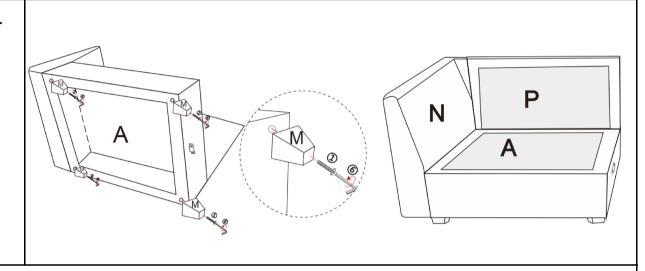
Lay Left Seat Board (A) flat, align Leg (M) with the holes at the bottom of Left Seat Board (A), and use Allen Wrench (⑥) to tighten Single Head Screw (①). This step tightens Single Head Screw (①).
