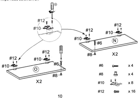
Step 15. Attach doors (parts N & O) with full curve hinges (part #10) to assembled unit (parts C, D & E) using phillips head screwdriver.
