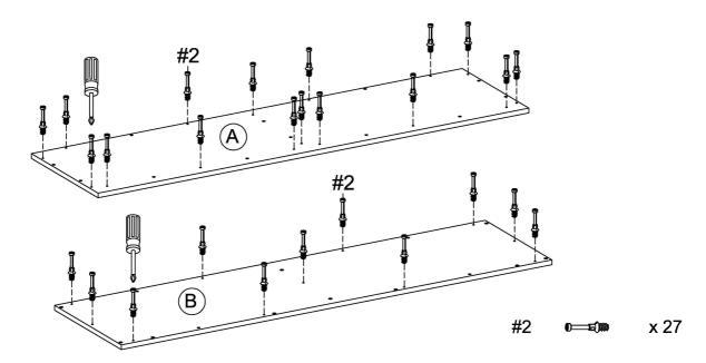
Step 2. Screw cam bolts (part #2) into left panel (part C) and right panel (D) using phillips head screwdriver.
