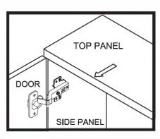
STEP 2 Adjust the gap between door panel and side panel
