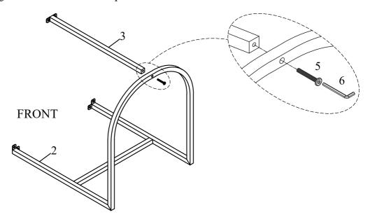
STEP 2 Attach Front Leg Frame (2) and Back Leg (3) to the bottom of Stool back with seat (1) with bolts (4) using Allen key (6).
