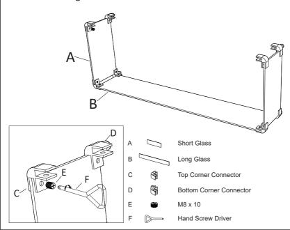
**Step4:**Fasten the other long piece of glass(B) with screws(E) on the top corner connector(C) and the bottom corner connector(D).
