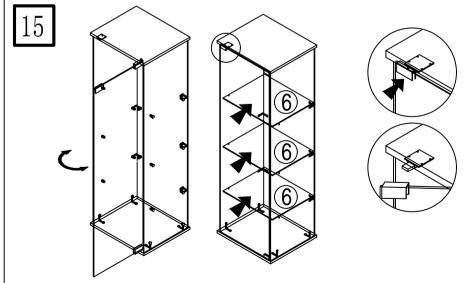
Put the glass shelf board into the main body while tilting it diagonally and place it on the dowel.
