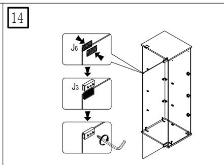
Use magnet [J3] and cushion [J6] to tighten screws to fix.
