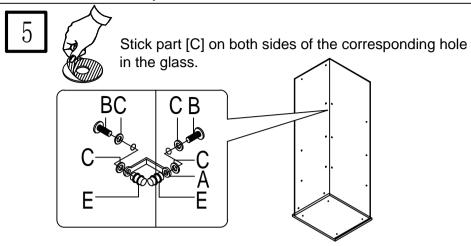
In the screw hole of the glass (side) Fixing parts [A], Temporarily tighten with dowels [E] .
