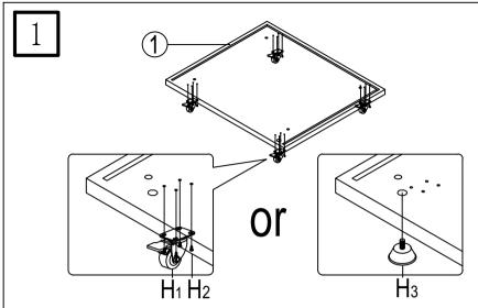
Option 1: Attach the wheel parts [H1] to [①] base plate. Option 2: Attach the foot parts [H3] to [①] base plate.
