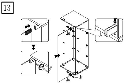
Door receiving metal fitting (lower part) [J1] cushion [J6] and Door receiving metal fitting (upper part) [J2] cushion [J6] Slide and insert, tighten screws to fix.
