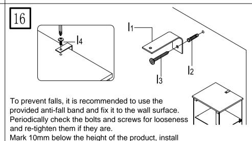
Place the product on the wall while pulling the attached anti-fall band
