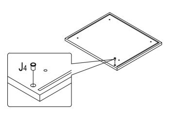
Attach the door holder [J4] to the [1] base plate.
