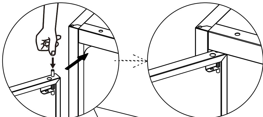
If you can't find the top hinge spring, it may have been pressed into the door frame. Simply use a screwdriver to gently pry it out.
