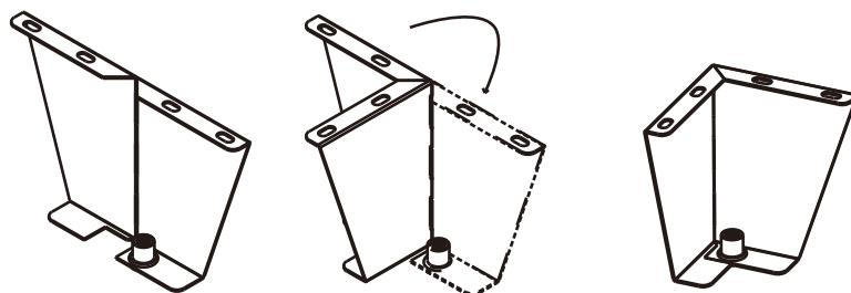
Manually bend the standing foot into shape and twist the adjustable foot in.
