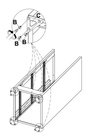
Put twelve screws to hold part C into place
