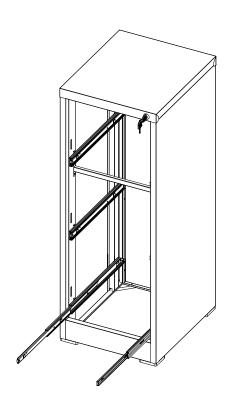
1.Pill out the small rails in the slide rails on the side walls completely. with two people lifing each side of the drawer, align the four divots on the bottom with the two rail clips on the rails on each side and insert them into the rail clips 2.After placing the drawer on the rail ,press the drawer base down hard enough, paying attention to check the position of the four clips inside until you hear a click four times, which means the drawer is in place
