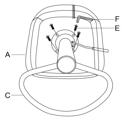
Insert the Gas Lift (D) to the Leg (C) as shown in below diagram. STEP 3
