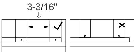
Note: Do not lock the screws of the bed slats to the outermost edge the bed slats, you need to leave a certain space at the edges, otherwise it will cause the board to break.
