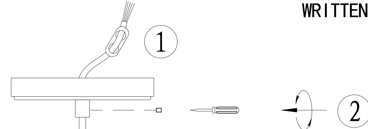
Adjust the wire to demand length by adjusting the plastic cable piece.
