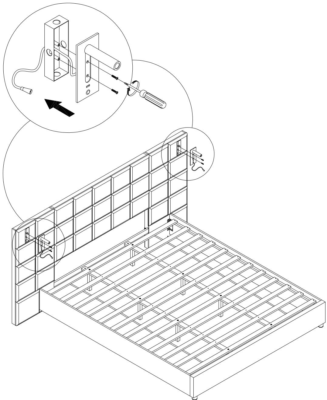
Attach the remaining part of the light (H) as before. Be sure to thread the light wire behind two headboards (2A) and (2B).
