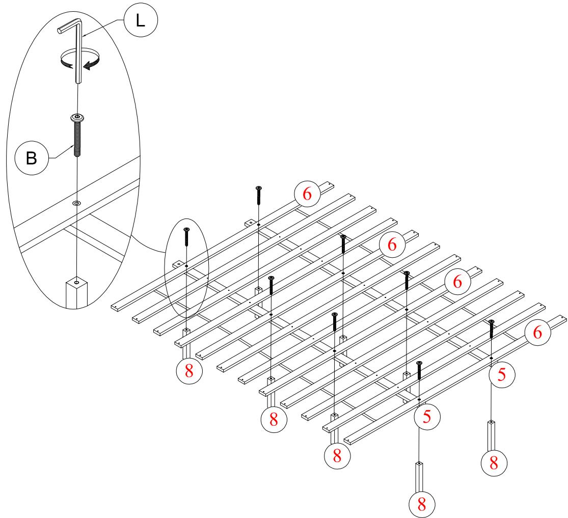
Align the Mounting Position on the Slat Support Bar (5) to the Support Leg (8) and the Slat (6). Attach the Slat (6) and the Slat Support Bar (5) to the Support Leg (8) and by using 8 Bolts (B), with Allen Wrench (L).
