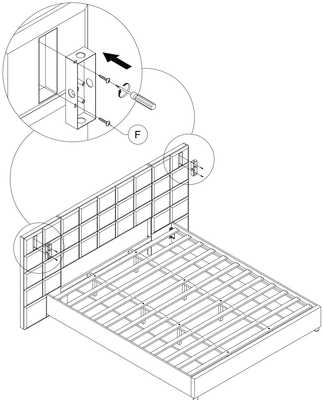
Attach the light box (removed from step 9) to the Left Headboard(2A) and Right Headboard(2B) by using 4 Screws (F) and a Screwdriver (not provided).
