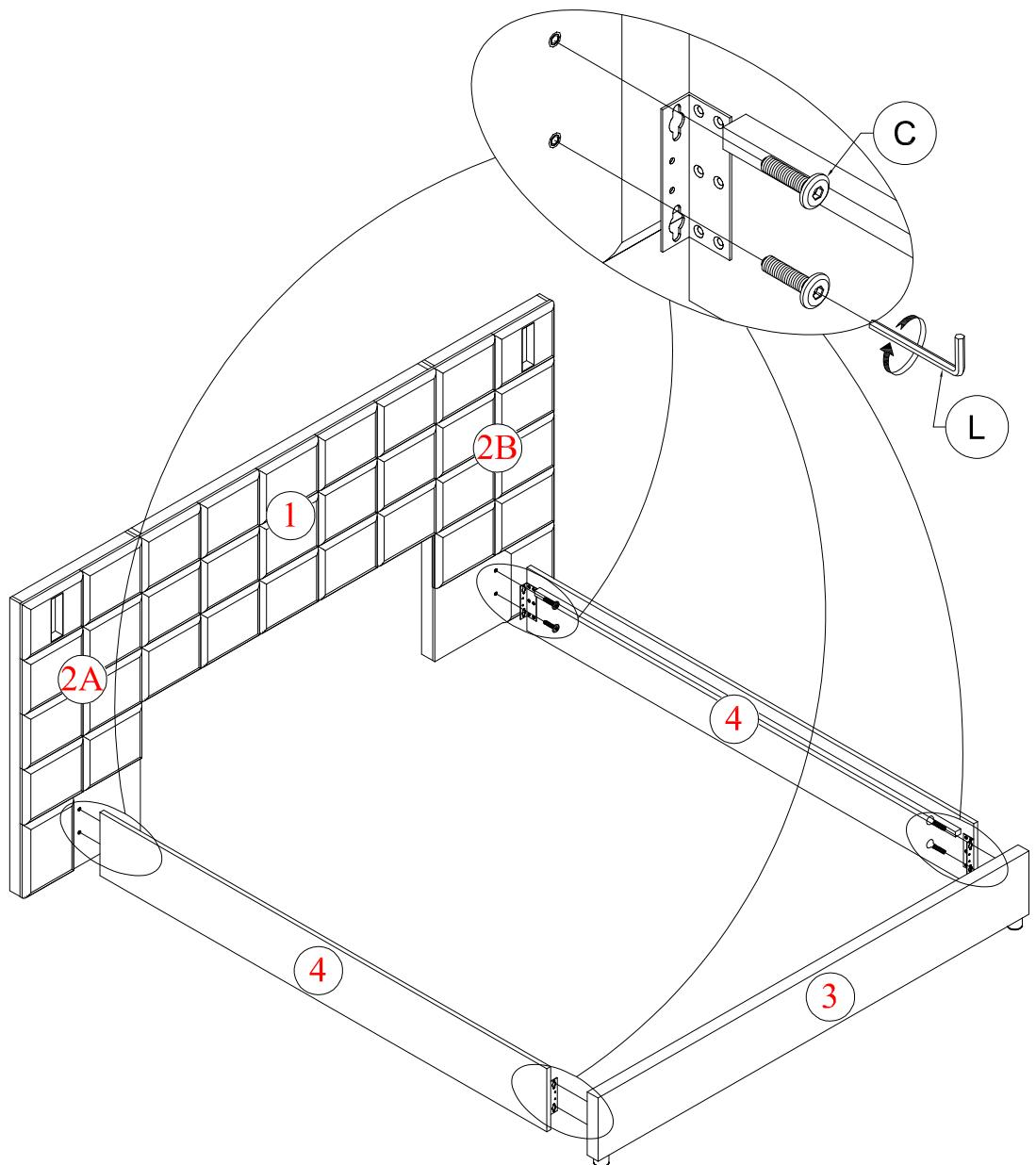
With the help of your partner, stand the completed the Footboard (3) from Step 2 and Headboard from Step 3 as shown in the picture above. Affix the Side Panels (4) to the Headboard (2A & 2B) and Footboard (3) using 8 Bolts (C) with Allen Wrench (L).
