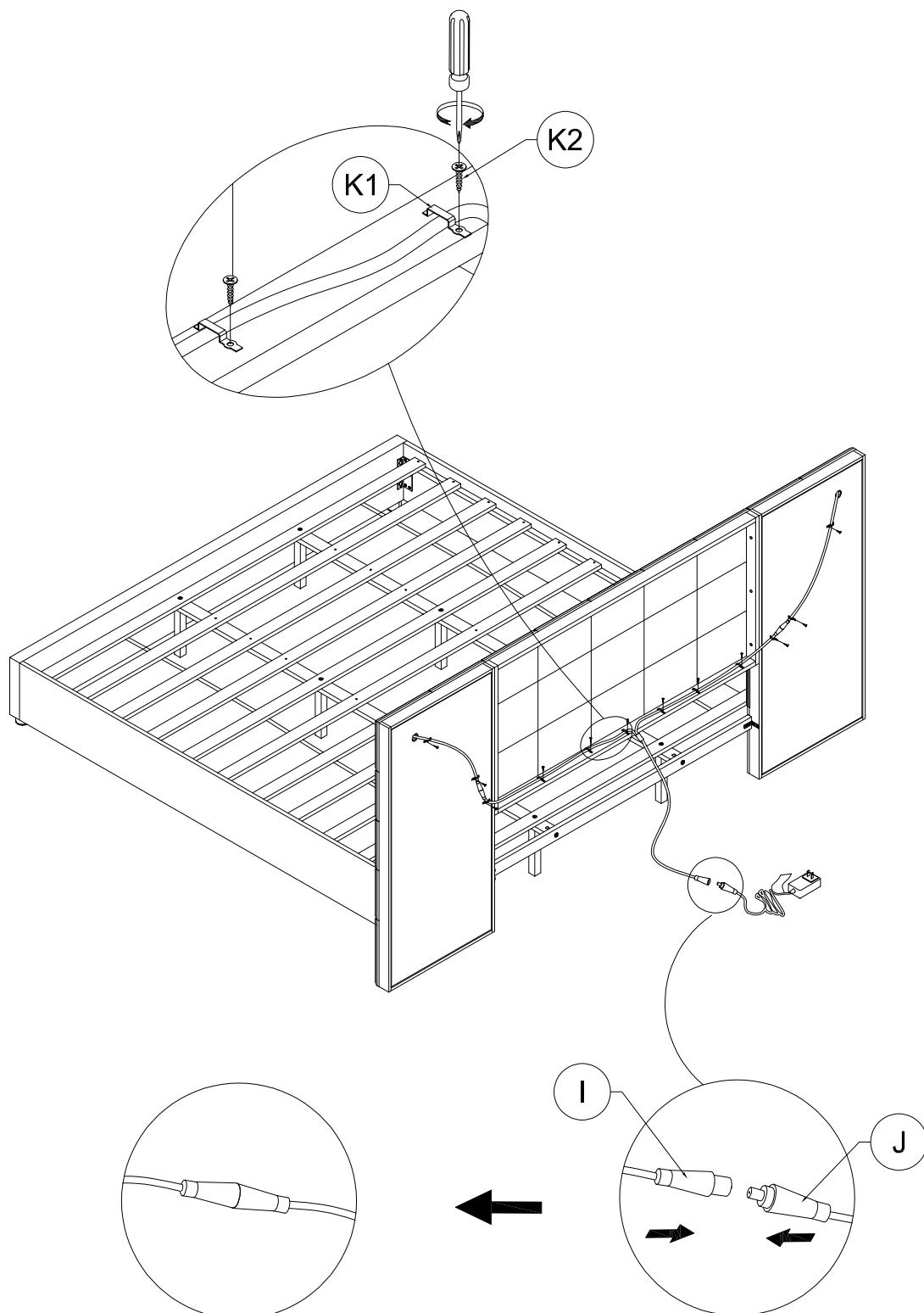
Connect the connection cable (I) to the Apdapter (J).
