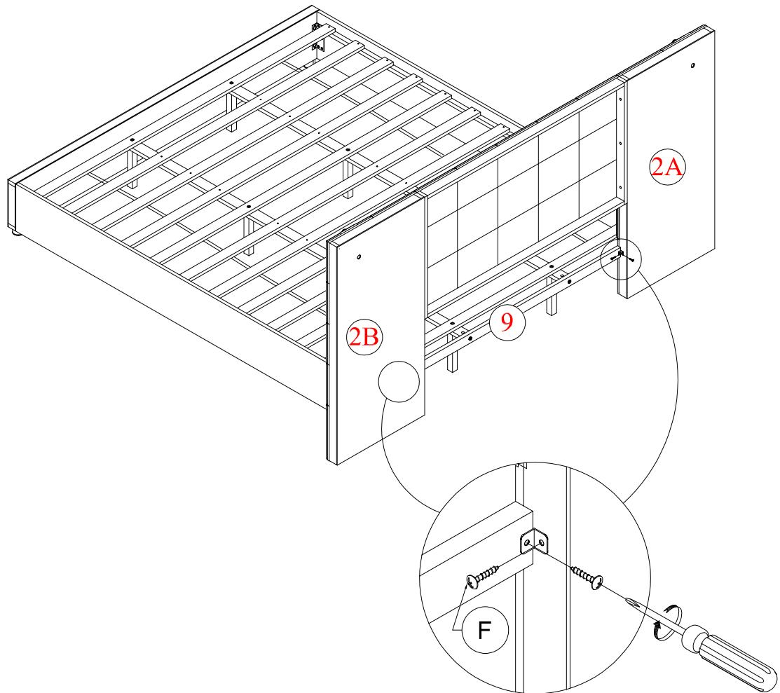
Fix the Horizontal bar (9) to the Left Headboard (2A) and Right Headboard (2B) by using steel bracket (G), Screws (F) and a Screwdriver (Not Provided).
