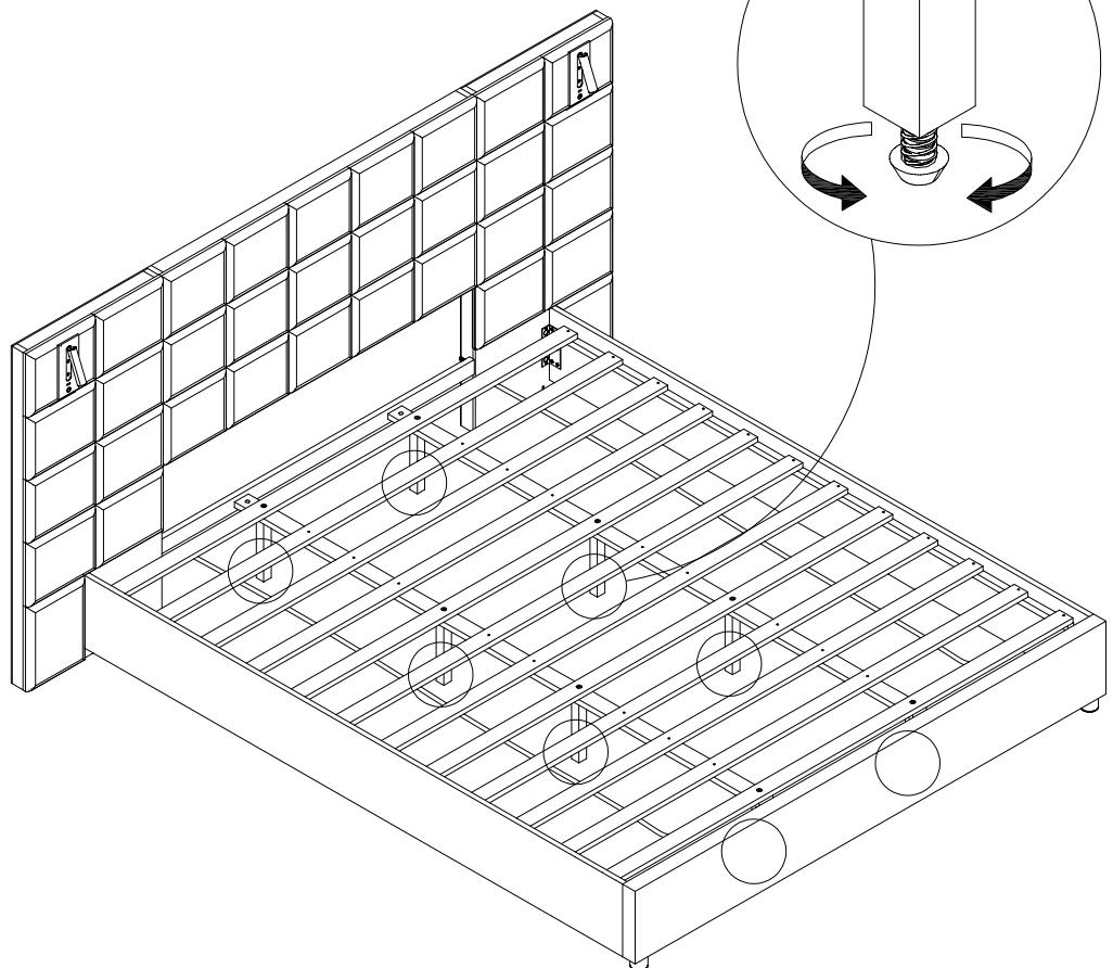
Rotate counterclockwise to increase the length of Floor Leveler, and raise that corner.
