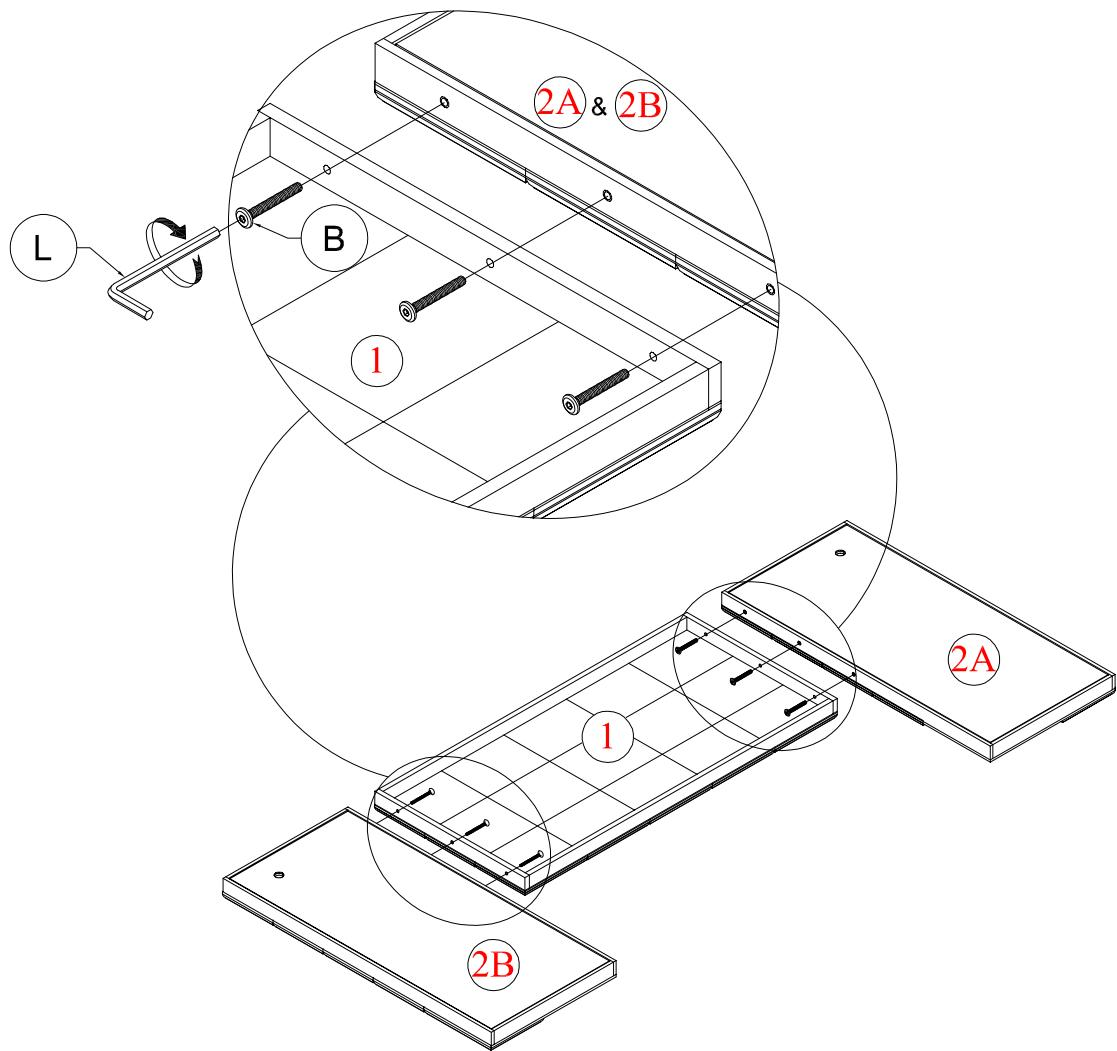
Align the Mounting Position of Left Headboard (2A) and Right Headboard (2B) into the Mounting Position of Center Headboard (1) as shown above. Affix to Center Headboard (A) by using using Bolts (B) with Allen Wrench (L).
