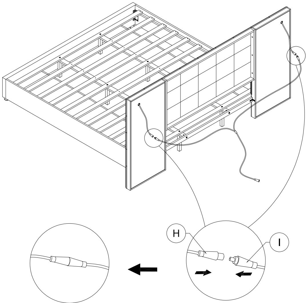
Connect the light wire (H) to the connection cable (I).
