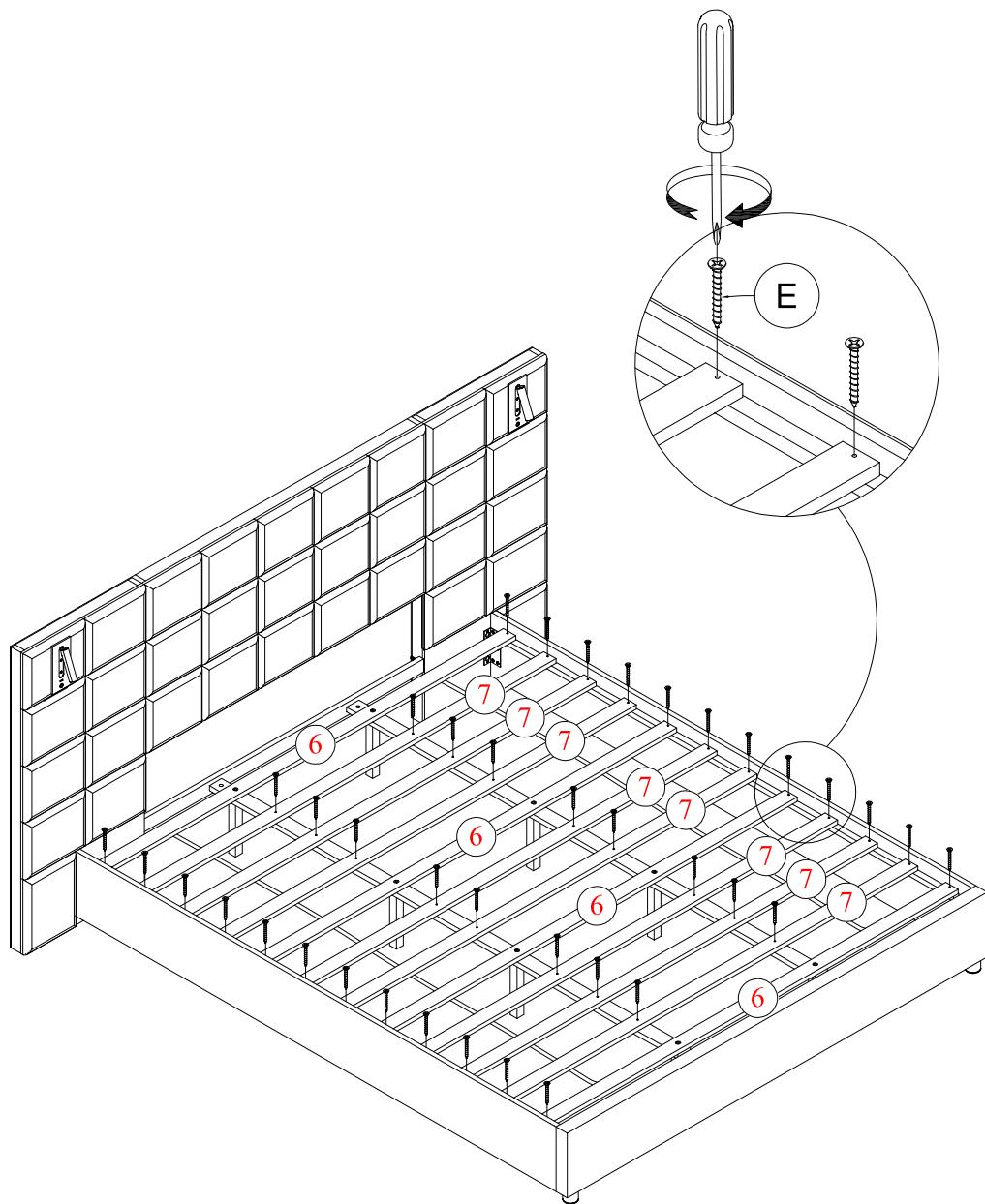
Attach all Slats (6), (7) to the rail on Side Rails (4) by using 40 Screws (E) and Screwdriver (Not Provided).
