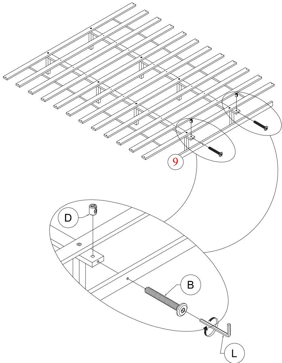
Align the Mounting Position on Horizontal bar (9) to the Slat Support Bar (5). Attach Horizontal bar (9) to the Slat Support Bar (5) by using 2 Bolts (B), 2 Horizontal - Hole Bolt (D) with Allen Wrench (L).
