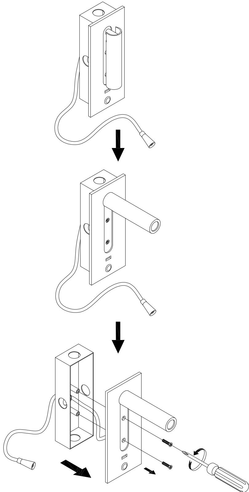
Use a Screwdriver (Not provided) to open the Light box (H) . Be careful not to lose any parts of the light.
