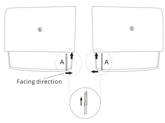
Step4 Connect 6 and 5 to 1,2,3 and 4 as a whole through the Latch slider.
