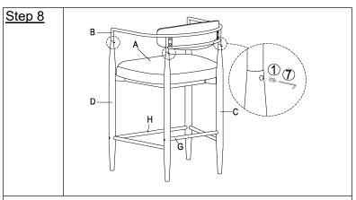
Using Bolts(①) with the Allen Wrench(⑦) affix together the Backrest (B), the Left Metal Leg Frame(C) and the Right Metal Leg Frame(D) as shown above.
