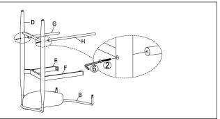
Attach the Back Bottom Rail(G) and Footrest(H) to the Right Metal Leg Frame(D) using the Bolts(②), with the Allen Wrench(⑥) as shown above.
