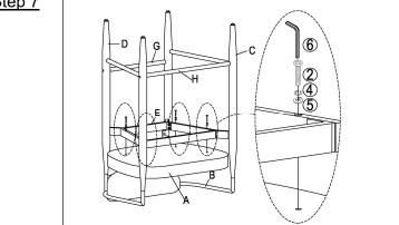
Position the Seat(A) (bottom-up) as shown above, then using Bolts(@), Spring Washers(4), and Washers (5), with the Allen Wrench(6) affix the Seat(A) to the Left Metal Leg Frame(C) and Right Metal Leg Frame(D).
