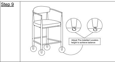
Adjust the Pre-installed Levelers at the bottom of the Left Metal Leg Frame(C) and Right Metal Leg Frame(D) until the Counter Stool is level with the ground.
