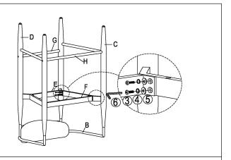
Using Bolts(③),Spring Washers(④), and Washers (⑤), with the Allen Wrench(⑥) affix together the Left Metal Leg Frame(C), the Back Upper Rail(E) and the Front Upper Rail(F) as shown above.
