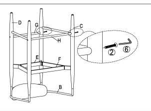
Using Bolts(2) with the Allen Wrench(6) affix together the Left Metal Leg Frame(C), the Back Bottom Rail(G) and the Footrest(H) as shown above. Note: Do not fully tighten the Bolts in this step.
