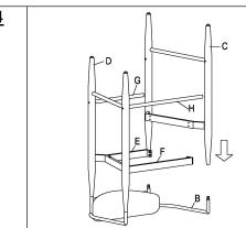
Insert the Left Metal Leg Frame(C) onto the Backrest (B) as shown above. Note: Do not fully tighten the Bolts in this step.
