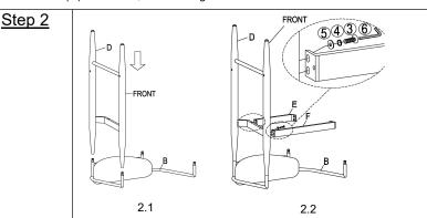
2.1 Place the Backrest(B) facedown on a clean, non-marring surface. Insert the Right Metal Leg Frame(D) onto the Backrest(B). 2.2 Attach the Back Upper Rail(E) and Front Upper Rail(F) to the Right Metal Leg Frame(D) using Bolts(③), Spring Washers(④) and Washers (⑤), with the Allen Wrench(⑥) as shown above.
