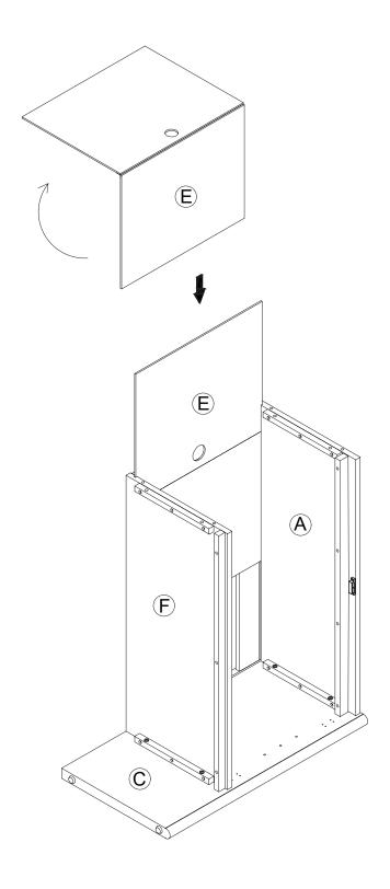
Next, insert the Wooden Dowels (3) into the Top Panel (A) & Bottom Panel (F), then attach it to the Side Panel (Left) (B) using the Flat Washers (5) and Bolts (4).
