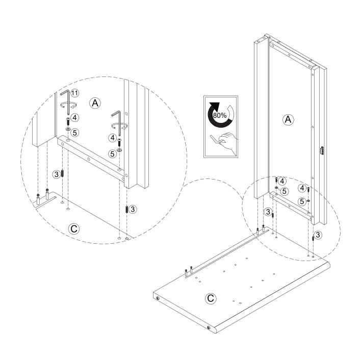
Next, insert the Wooden Dowels (3) into the Right Side Panel (C), then attach it to the Bottom Panel (F) using the Flat Washers (5) and Bolts (4).
