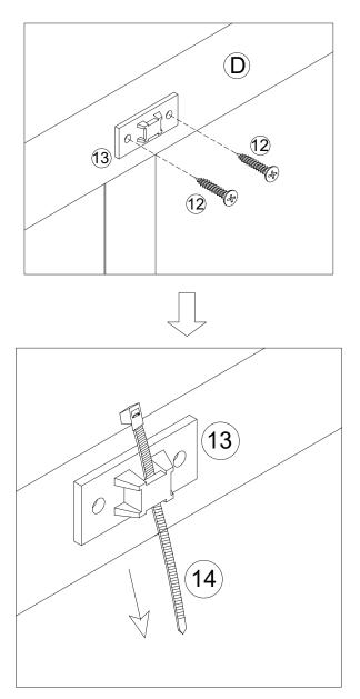
Find where you want your storage unit to live and then mount the Plastic Bracket (13) to the wall using the provided Wall Anchors (15) and M4\*35mm Screws (16). We recommend using a 1/4" drill bit.
