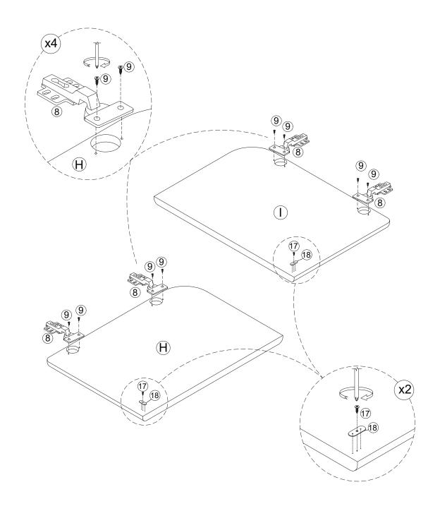
It's all coming together! Secure the doors to the unit by the Hinges using the M4 x 19mm Screws (9).
