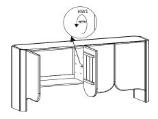
5. Now tilt the shelf (A) and insert it and place the shelf on top of the pins (HW1).
