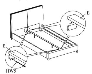
ATTENTION: Please ensure that (HW5) screw are being attached as the AI shows to avoid the base collapsing.
