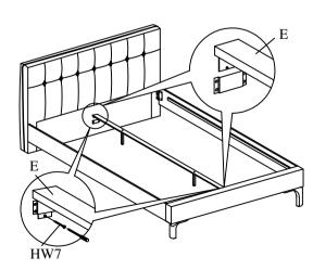
ATTENTION: Please ensure that (HW7) screw are being attached as the AI shows to avoid the base collapsing.
