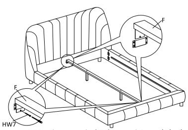
ATTENTION: Please ensure that (HW7) screw are being attached as the AI shows to avoid the base collapsing.
