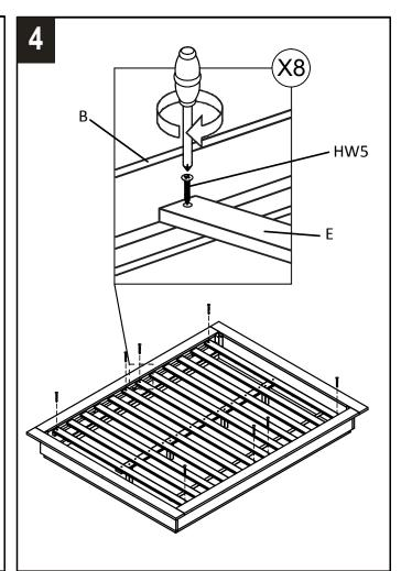
**STEP 4:** Place the assembled slat roll onto the assembled bed frame. Use the Philips head screwdriver to screw in the Screws (HW5) into the 8 holes on the siderails as shown.
