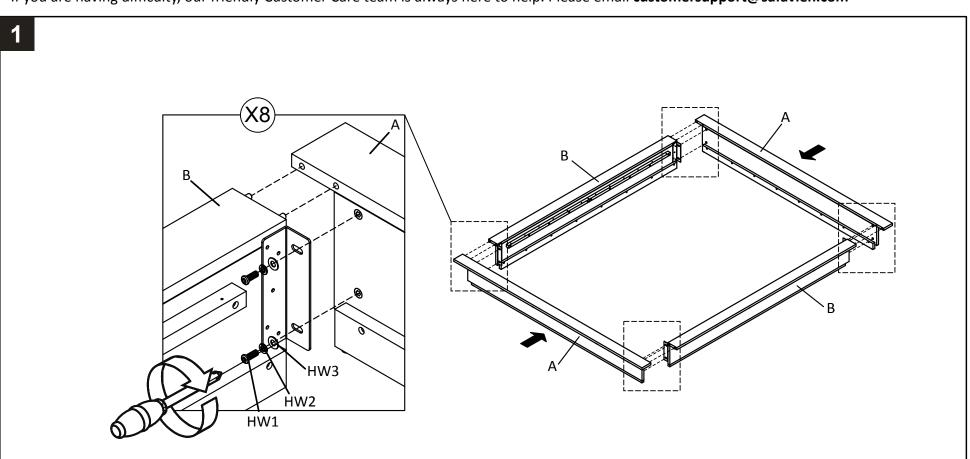
STEP 1: Place the split lock washer (HW2) and the flat washer (HW3) on the Philips head bolt (HW1) as shown.
