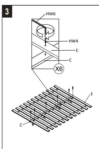
STEP 3: Attach the slat roll (E) to the center slat (C) by aligning the holes on the slat roll to the 1st, 3rd, 5th, 6th, 8th, and 10th pre drilled holes in the center slat.
