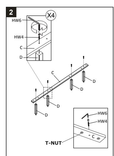
STEP 2: Place the center slat (C) with the T-nuts facing the floor. Put the Allen bolts (HW4) into the 2nd, 4th, 7th, and 9th predrilled holes in the center slat. Use the Allen Key (HW6) to screw in the Allen bolts (HW 4) into the support legs (D) as shown.
