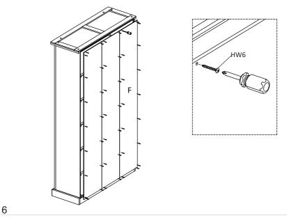
To help prevent the possibility of tipping over, install the tip over restraint kit provided.
