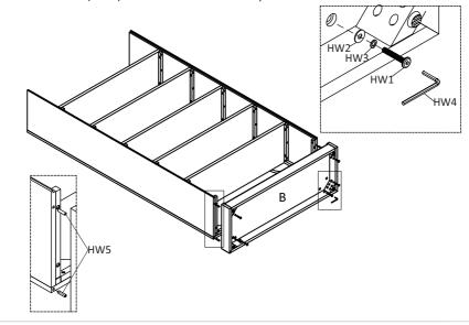
Insert one end of the Dowels (HW5) into the top of the assembled shelves and the other end into the top panel (A). Place the Spring Washers (HW3) and Flat Washers (HW2) on the Bolts (HW1). Attach the assembled shelves to the top panel (A) by using the Allen Key (HW4) to screw in the Bolts (HW1) with the washers in the spots shown below.
