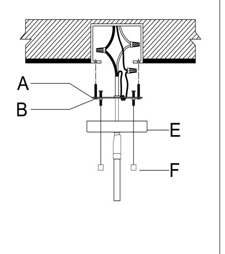
**Step 4:** Fix the Mounting Plate(A) to the junction box with Mounting Screw (B).
