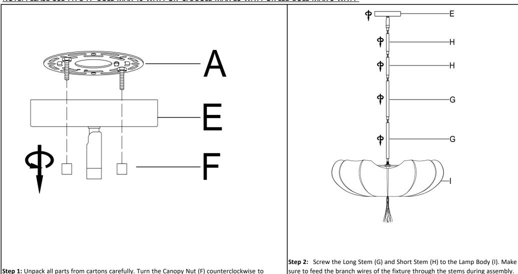
separate the Mounting Plate (A) and Canopy (E)
