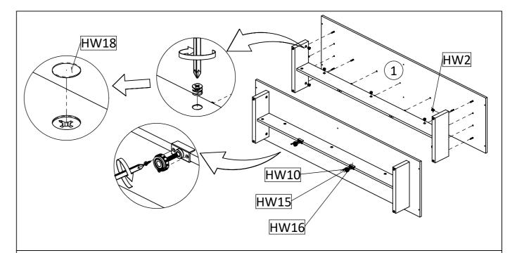
STEP4: Insert leg (2) and leg support (3)into bottom panel (1) Secure with Camlock big (HW2).Continue by attaching , plastik "U" (HW16) to position as picture above, using M6x12mm screw (HW10). Continue by attaching, adjuster (HW15) to position as image above, rotate and adjust. Attach Cover Cap Sticker (HW18) to the panel that has lamination.
