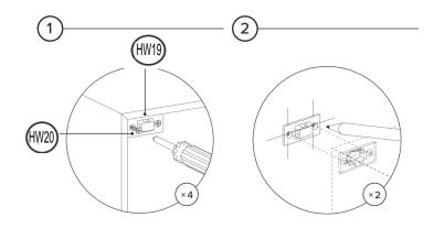
Attach pair of brackets to "Top Panel" of the unit. Note there are no existing pilot holes on the product.
