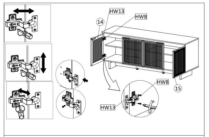
STEP17: Attach straight hinge (HW13) into left door (14) And right door (15), using M5x12mm screw (HW8) and tighten it using screwdriver.
