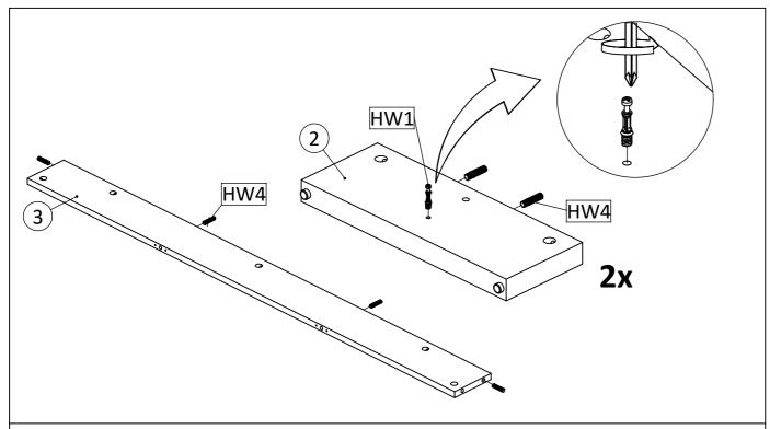
STEP1: Insert Cambolt (HW1) into leg (2) .Insert Wooden Dowel Big (HW4) into leg (2) and leg support (3).
