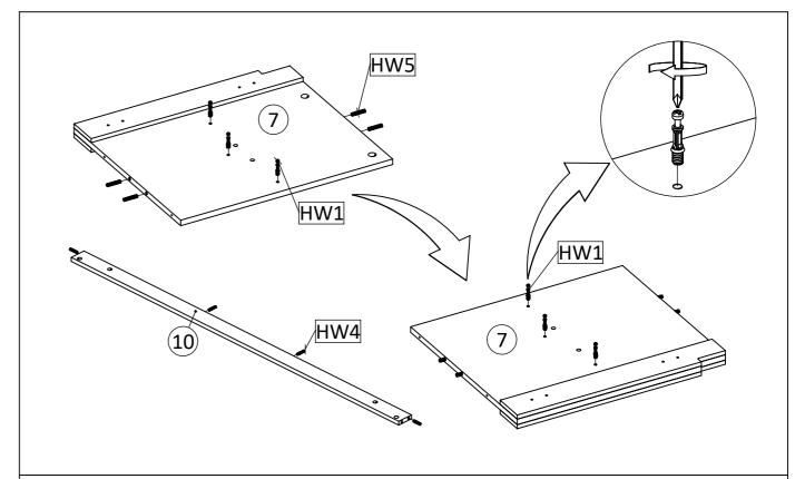
**STEP8:** Insert Cambolt (HW1) into center panel (7) insert Wooden Dowel small (HW5),into center panel (7) and insert Wooden Dowel big (HW4) into top support (10).
