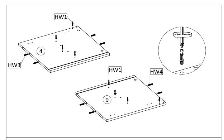
**STEP7:** Insert Cambolt (HW1) And Wooden Dowel big (HW4) Into left side panel (4) and right side panel (9).
