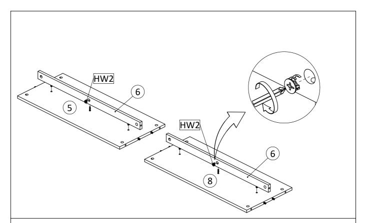
**STEP6:** Attach support middle panel (6) Into left fixed shelf (5), and into right fixed shelf (8). Secure with Camlock big (HW2) Tighten It Using Screwdriver.
