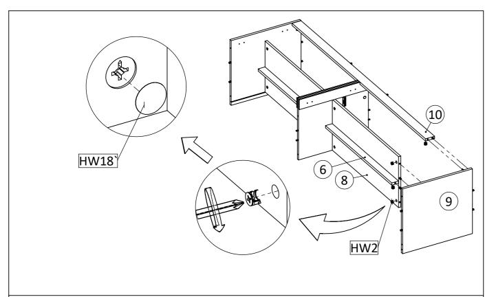
**STEP11:** Attach right side panel (9), into support middle panel (6), right fixed shelf (8) and top support (10) Secure with Camlock big (HW2). Attach Cover Cap Sticker (HW18) to the panel that has lamination.
