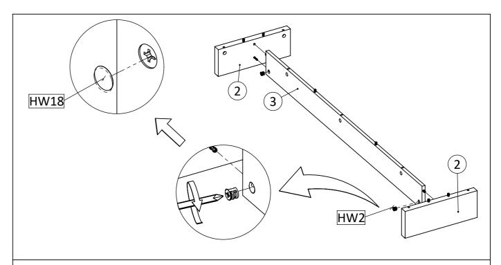
**STEP 2:** Attach leg (2) into leg support (3), Secure with Camlock big (HW2) and tighten it using screwdriver. Attach Cover Cap Sticker (HW18) to the panel that has lamination.
