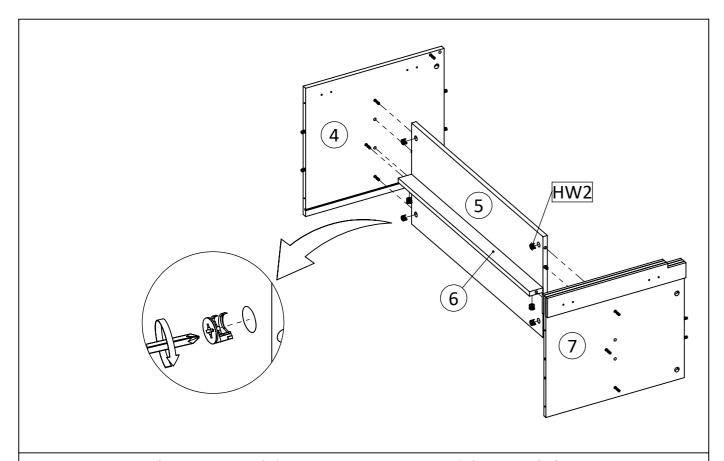
**STEP9:** Attach left side panel (4) and right side panel (7), into left fixed shelf(5) and into support middle panel (6) . Secure with Camlock big (HW2).
