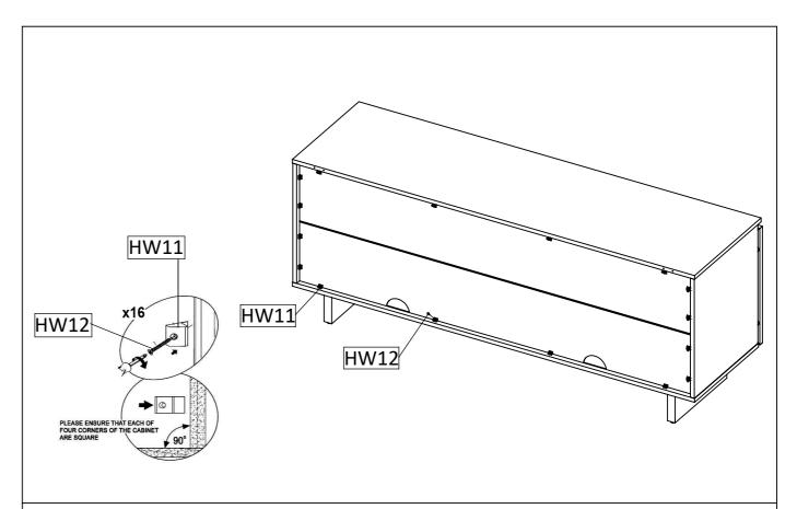
**STEP18:** Attach the plastic stopper (HW11) to upper back panel(11), and into lower back panel (12) Securewith screw M4x19 mm (HW12) and tighten it using screwdriver.
