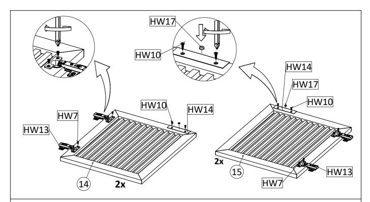
**STEP16:** Attach straight hinge (HW13) into left door (14) And right door (15), using M5x8.5mm screw (HW7) and tighten it using screwdriver. attach door handle (HW14) into left door (14) and right door(15), using screw 6 X 12 MM (HW10) and tighten it using screwdriver. Continue to install the rubber stopper (HW17) to the front side of the left door (14) and the right door (15).
