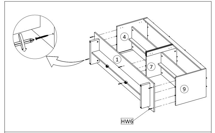
**STEP12:** Insert left side panel (4), center panel (7) and right side panel (9), into bottom (1). Secure with screw M6 X 50 MM (HW6).
