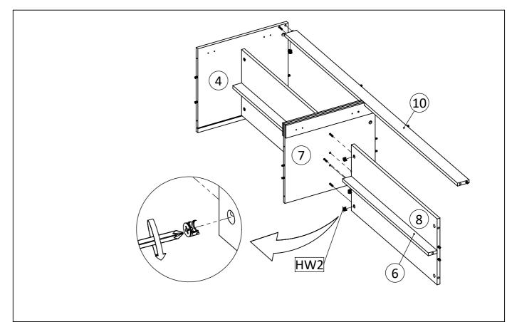
**STEP10:** Attach fixed shelf (8), support middle panel (6) into center panel (7), and attachright top support (10) into left side panel (4) Secure with Camlock big (HW2).
