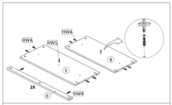
STEP5: Insert Cambolt (HW1) into left fixed shelf (5) and right fixed shelf (8). Insert Wooden Dowel Big (HW4) into left fixed shelf (5), right fixed shelf (8) and into support middle panel (6).
