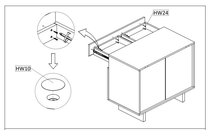
**STEP14:** Combine body drawer to front drawer (15) Secure with Sekrup M6x25MM (HW24) ,tighten it using screwdriver.Continue to attach the cover cap sticker (HW10) to the panel that has lamination.
