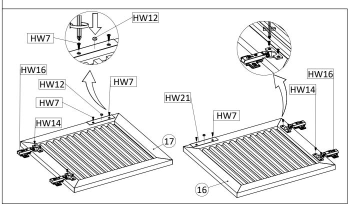
**STEP16:** Attach straight hinge (HW16) into left door (16) And right door (17), using M5x8.5mm screw (HW14) and tighten it using screwdriver. attach door handle (HW21) into left door (16) and right door(17), using screw 6x12 MM (HW7) and tighten it using screwdriver. Continue to install the rubber stopper (HW12) to the front side of the left door (16) and the right door (17).
