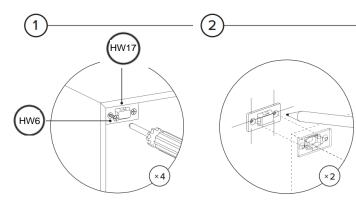
Attach pair of brackets to "Top Panel" of the unit. Note there are no existing pilot holes on the product.
