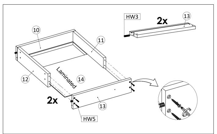
**STEP11:** Insert Wooden Dowel (HW3) into Side Drawers right (13), Combine Side Drawers right (13), Drawer back (11), drawer front support (12) and drawer base(14). then secure with Screw M7x32mm (HW5).
