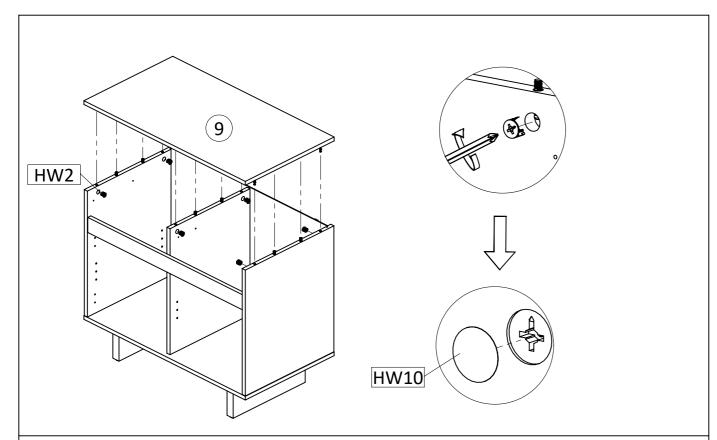
**STEP9:** Insert Top panel (9) Secure with Camlock(HW2), and tighten it using screwdriver. Continue to attach the cover cap sticker (HW10) to the panel that has lamination.
