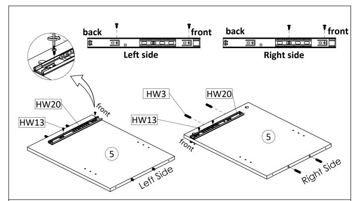
**STEP4**: Insert Wooden Dowel (HW3) into center panel (5), Continue with securing part of the metal runner 2 (HW20) into position as the above image, using screw M6x12mm PH (HW13).
