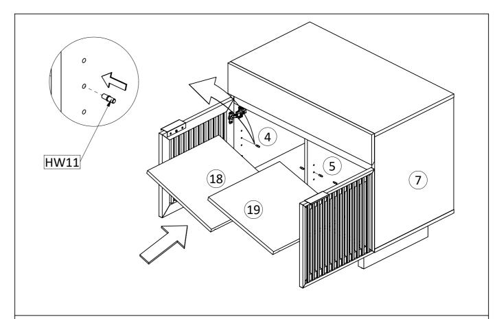
**STEP18**: Insert the metal pin (HW 11) into the left panel (4), right panel (7) and center panel (5), Insert Adjustable shelf-left (18) and Adjustable shelf-right(19), into body
