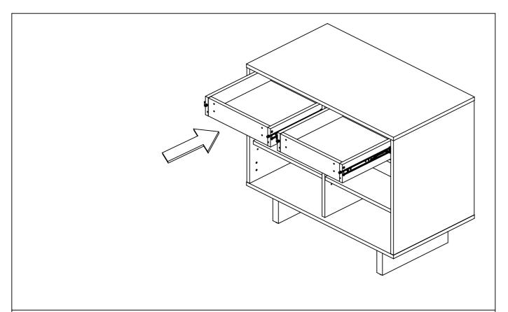
**STEP13:** Hold the sides of drawer, position the wheel of rail at drawer back and the wheel of rail at side boards, according to the image. Slide in the drawers into the cabinet.
