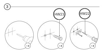
Drill holes in wall using 8mm / 5/16" drill bit.
