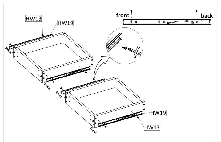
**STEP12:** Install the metal runner 1 (HW19). Secure with screw M6x12mm PH (HW13) And Tighten It Using Screwdriver.
