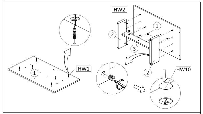
**STEP2:** Insert Cambolt (HW1) into bottom panel (1).insert leg (2) and leg support (3)into bottom panel (1) Secure with Camlock (HW2).Attach Cover Cap Sticker (HW10) to the panel that has lamination.
