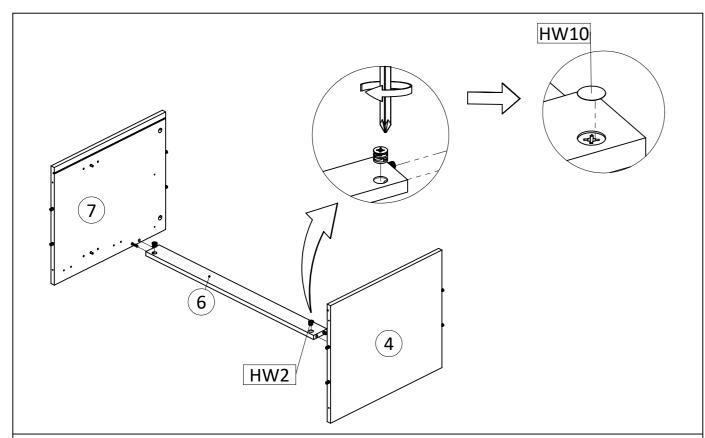
**STEP5:** Attach left side panel (4) and right side panel (7),into top support (6).Secure with Camlock (HW2).Attach Cover Cap Sticker (HW10) to the panel that has lamination.
