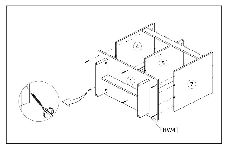
**STEP6:** Insert Left side panel (4), right side panel (7) and center panel (5), into bottom panel (1), Secure with screw M6 X 50 mm (HW4).
