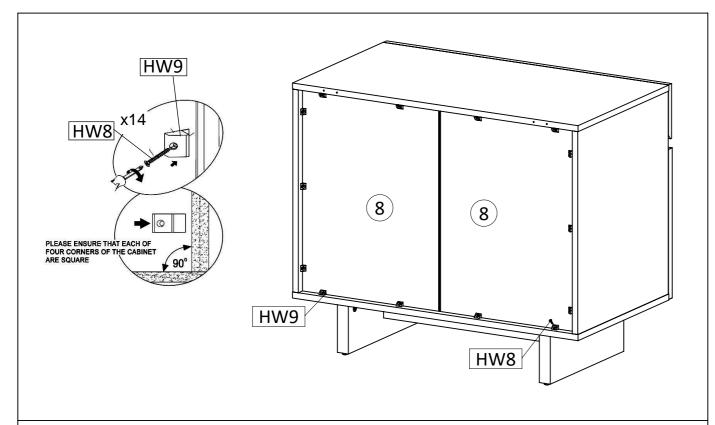
**STEP19**: Attach the plastic stopper (HW9) to the back panel (8), Secure with screw M4x19 mm (HW8) and tighten it using screwdriver.
