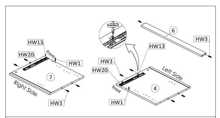
**STEP3:** Insert Cambolt (HW1) into left side panel (4) and right side panel (7).Insert Wooden Dowel (HW3) into left Side Panel (4) right side panel (7) and top support (6),Continue with securing part of the metal runner 2 (HW20) into position as the above image, using screw M6x12mm PH (HW13)
