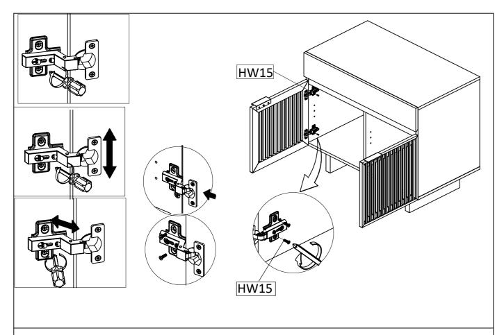
STEP17: Attach straight hinge (HW16) into left door (16) And right door (17), using M5x12mm screw (HW15) and tighten it using screwdriver.
