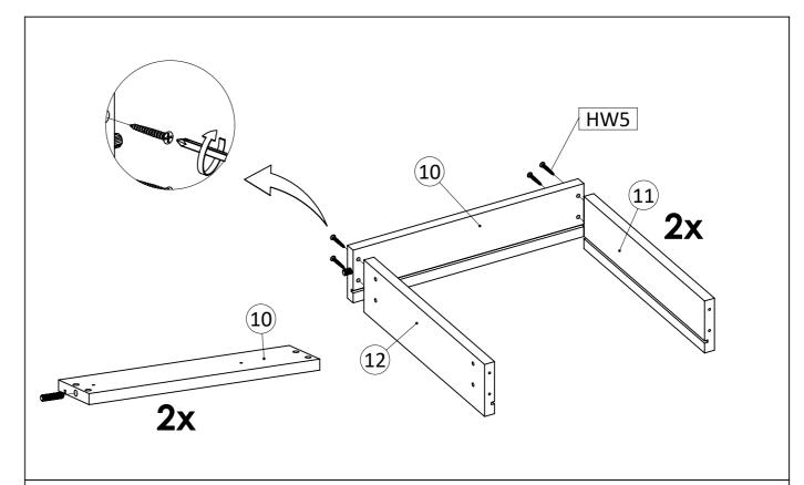
STEP10: Insert Wooden Dowel (HW3) into Side Drawers left (10), Combine Side Drawers left (10) Drawer back (11) and drawer front support (12). then secure with Screw M7x32mm (HW5).
