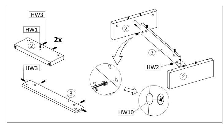
**STEP1:** Insert Cambolt (HW1) into leg (2) .Insert Wooden Dowel HW3) into leg (2) and leg support (3).Attach leg (2) into leg support (3),Secure with Camlock (HW2) and tighten it using screwdriver.Attach Cover Cap Sticker (HW10) to the panel that has lamination.
